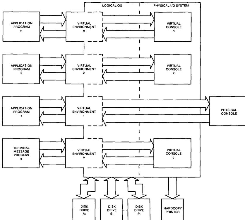
Figure 1-1. Concurrent CP/M Virtual/Physical Environments
