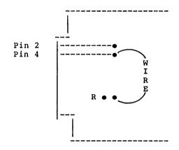
The SBC 204 Diskette Controller is jumpered by installing the following connections:
