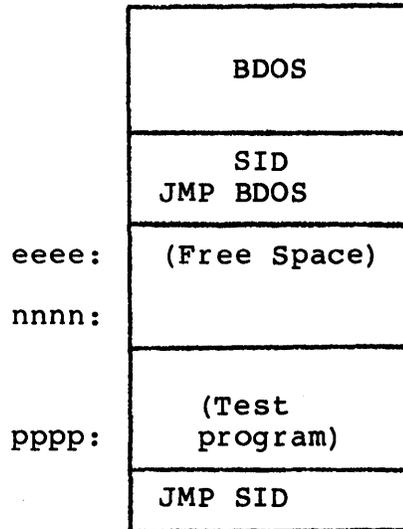
**Figure 1-3. Memory Configuration After Test Program Load**
