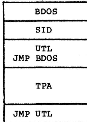
**Figure 1-4. Memory Configuration Following Utility Load**
