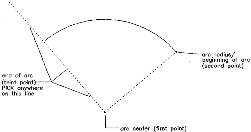
Figure 6-2. Drawing an Arc
