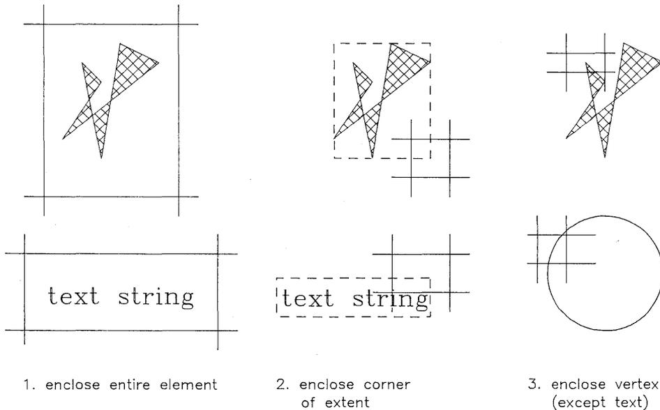
**Figure 5-13. Selecting a Current Element**
