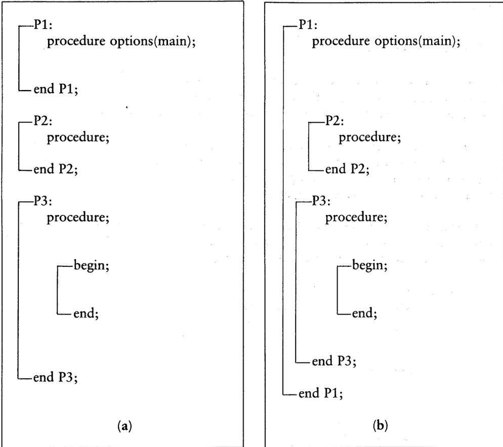
Figure 2-2. Internal and External Blocks
