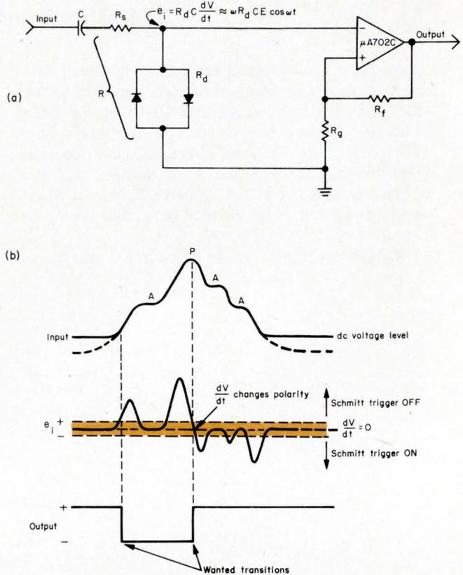
**Fig. 3. The improved peak detector (a)** is an op amp connected as a comparator. A clearly defined region between OFF and ON replaces the region of uncertainty in ordinary amplifiers. This eliminates spurious triggering, even in the presence of severe distortion. Diodes protect the comparator, and give the detector a large dynamic range.
