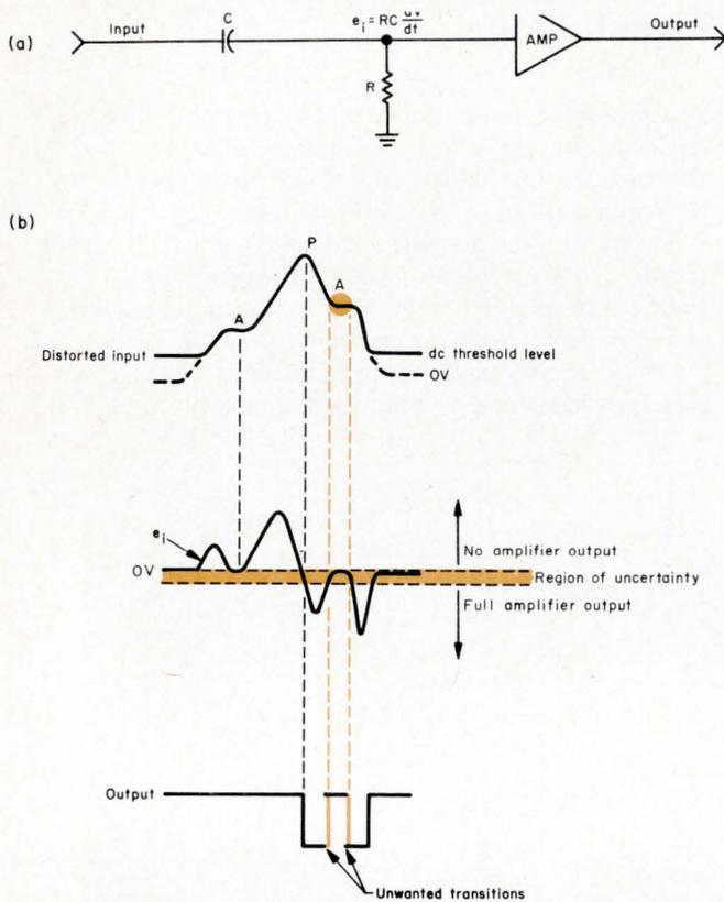
**Fig. 2. A conventional peak detector**, as in (a), consists of a differentiator,  $RC$ , followed by an amplifier. False zero-slope points,  $A$ , cause unwanted output transitions which are equivalent to erroneous binary ones. There is a limited dynamic range, and the amplifier's region of uncertainty causes spurious output transitions.
