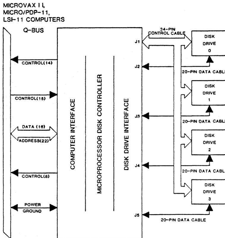
Figure 1-1. Disk System, Simplified
