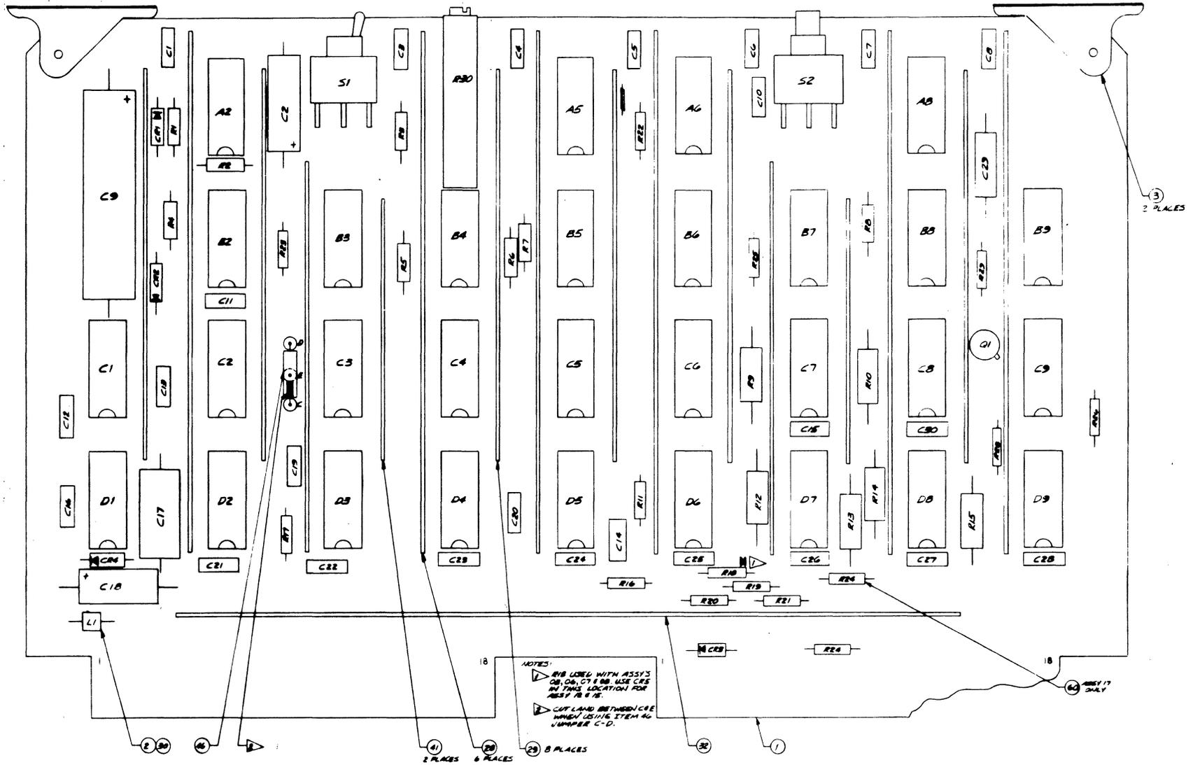
Figure 10-11. Assembly Diagram, Error Card
