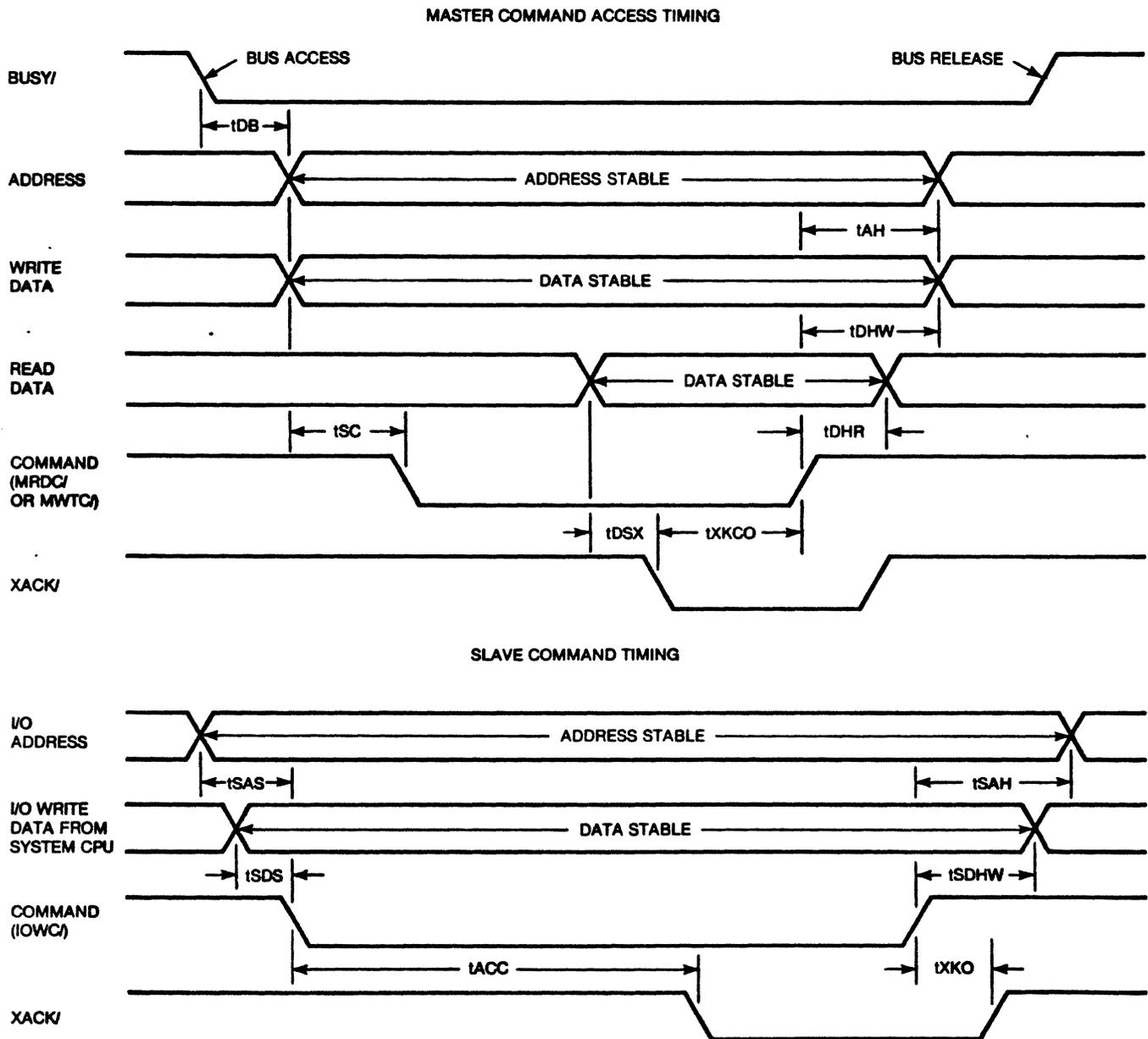
**Figure 2-2. Master Command Access Timing**
