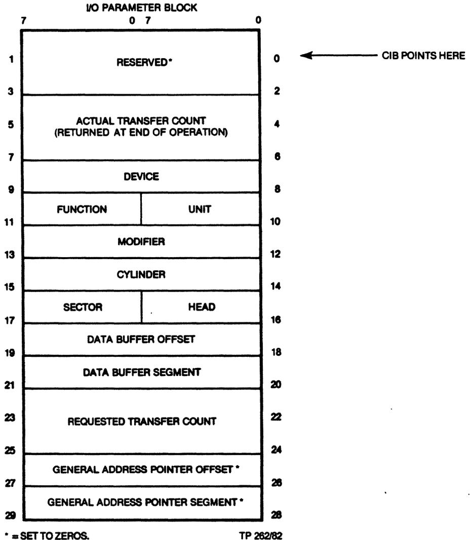
**Figure 4-7. Input Output Parameter Block**
