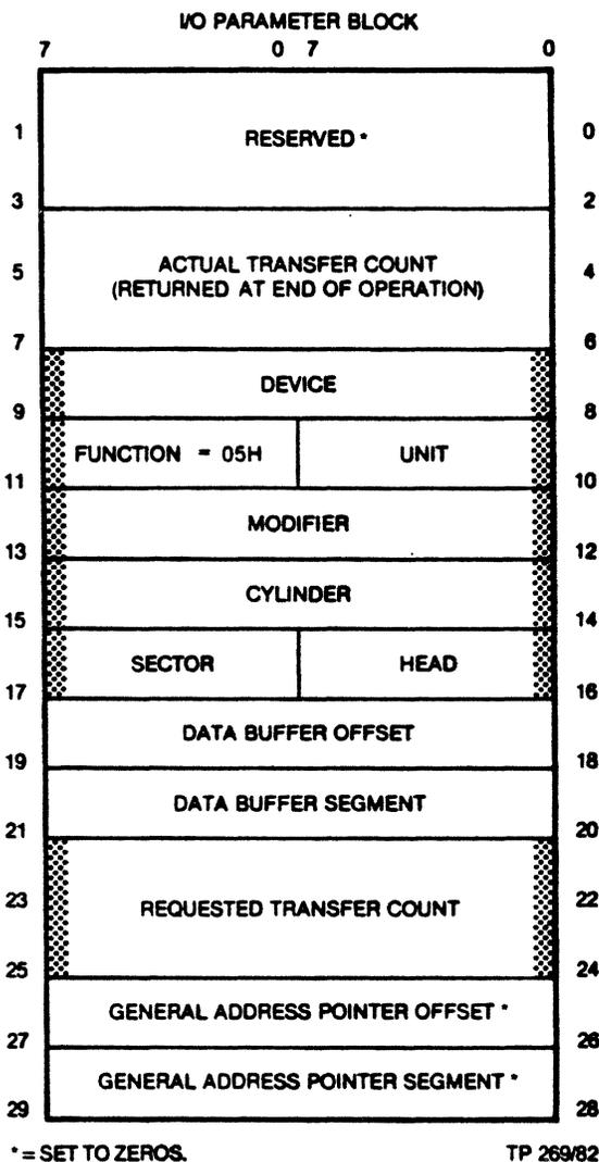
Figure 4-14. IOPB Read Buffer and Verify Function
