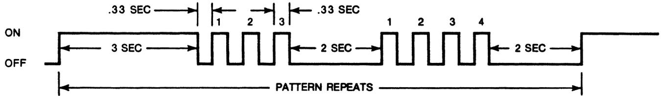
**Figure 6-2. CR1 Blinking Error Code**
