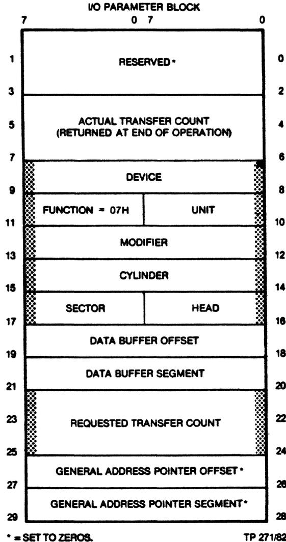
**Figure 4-16. IOPB Write Buffer Data Function**
