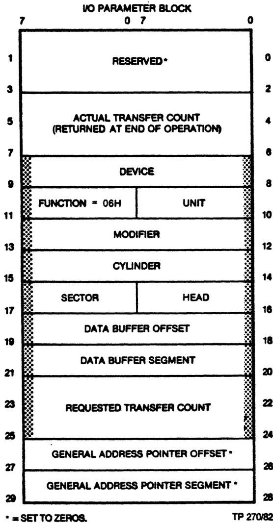
**Figure 4-15. IOPB Write Data Function**
