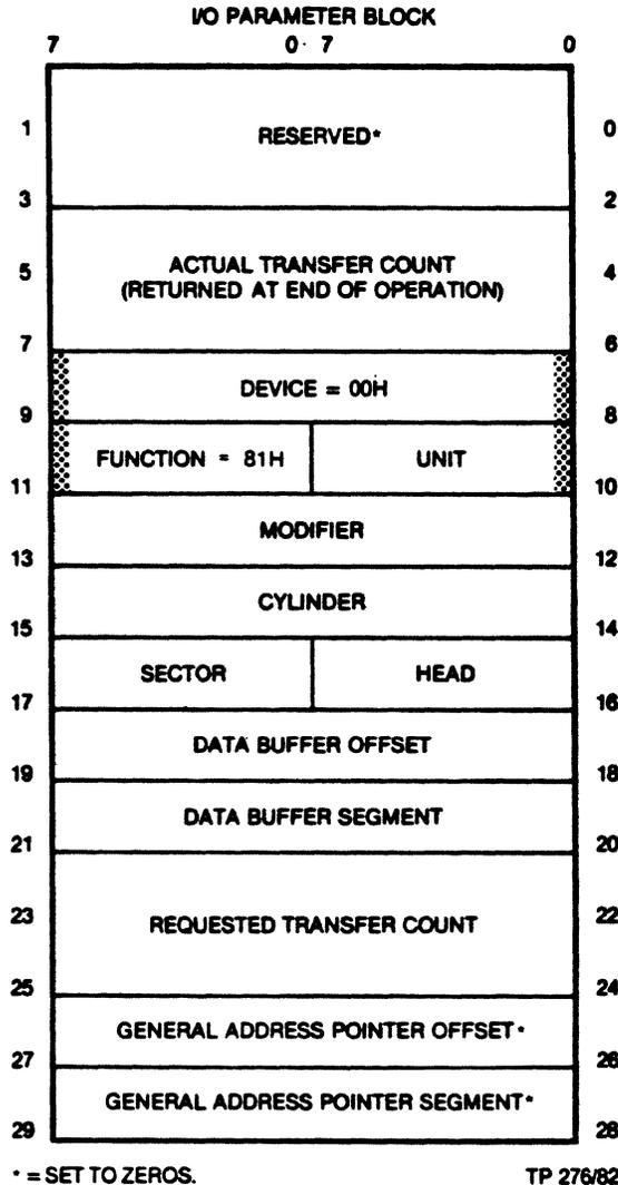
Figure 4-21. IOPB Disk Image Backup Function
