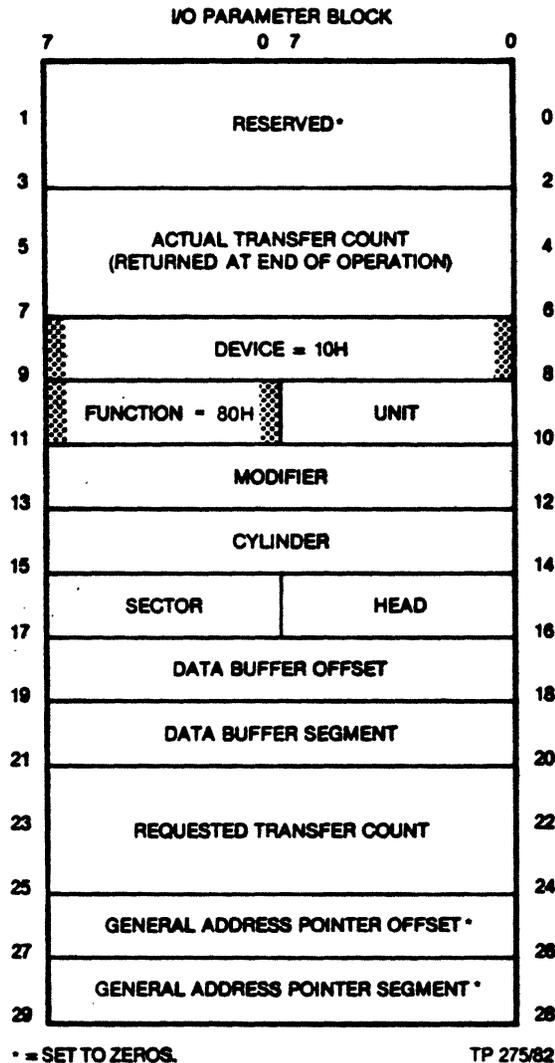
Figure 4-20. IOPB Reset Tape Drive Function
