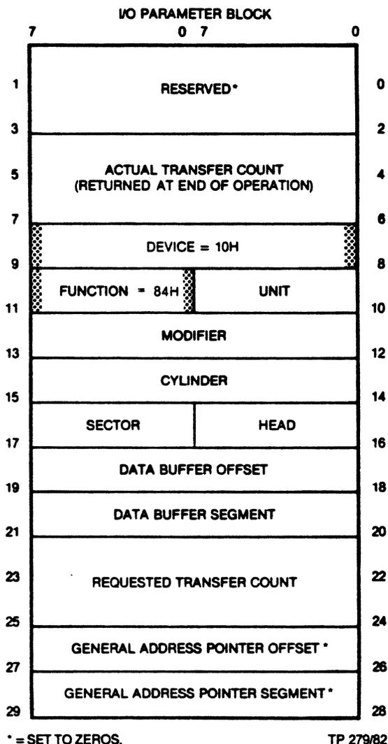
**Figure 4-24. IOPB Tape Retension Cycle Function**
