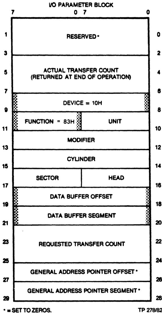
Figure 4-23. IOPB Read Tape Status Function
