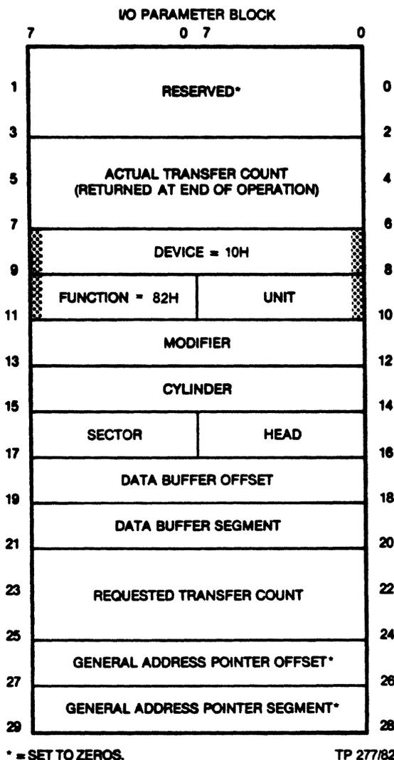
**Figure 4-22. IOPB Disk Image Restore Function**
