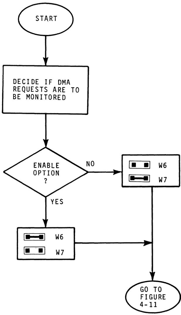
Figure 4-10. DMA Request Monitor Option TP 522/83
