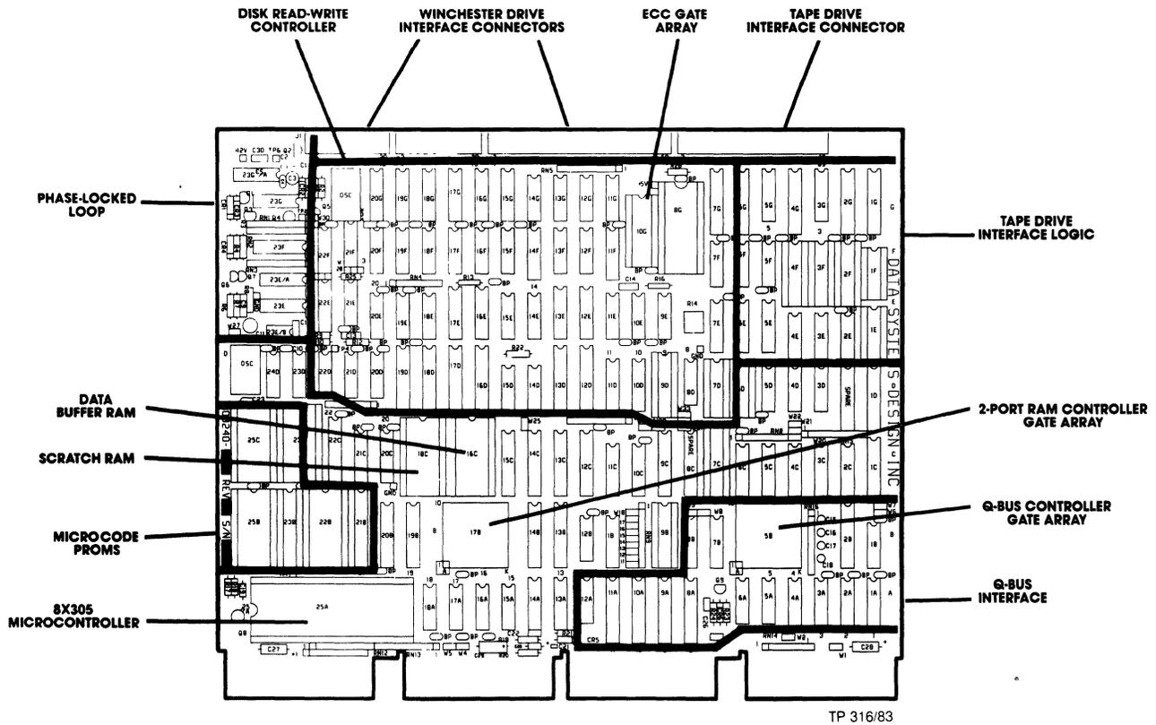
Figure 3-1. DSD 8240 Controller Board
