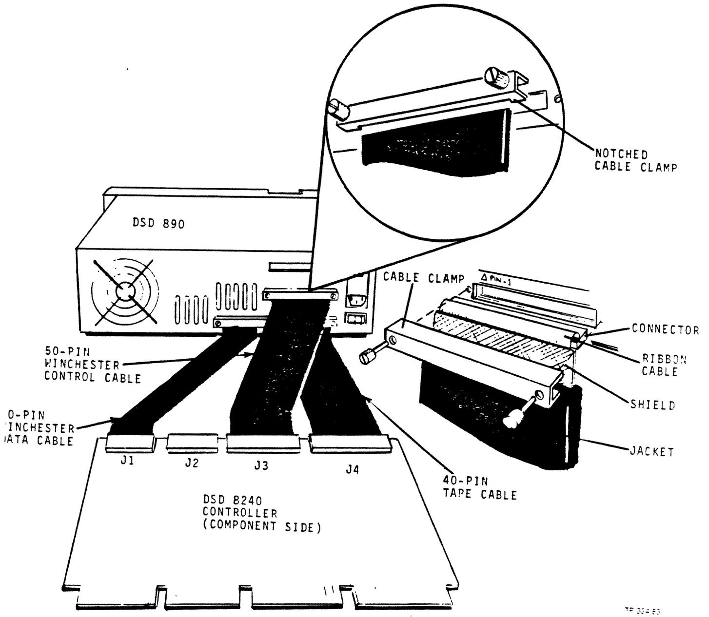
Figure 4-5. Cabinet and Board Cabling
