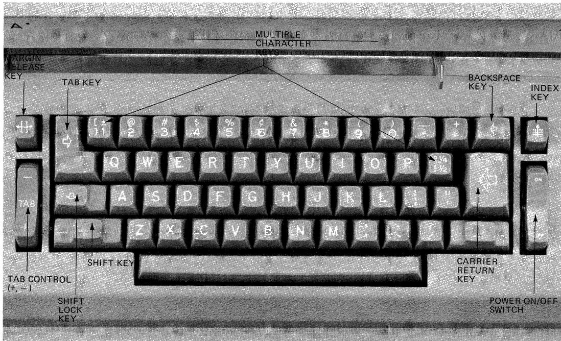
Typical keyboard for the Model 1021 series. Numerical keys and symbols may vary, depending on the particular model and the typing element selected.
