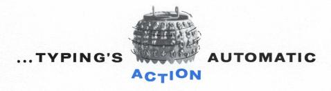
**PACESETTER:** The speed of the Mach 10 sets a new standard for high-production automatic typing. It reads punched paper tape automatically at approximately 175 words per minute. This speed, plus compatibility with other equipment, makes the Mach 10 the most productive automatic typewriter available. Additional Mach 10 "slave machines" will raise production to a frequency rate never before attained.
