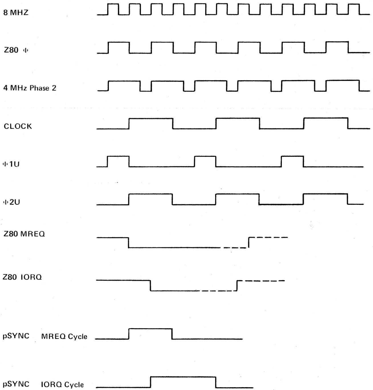
Figure 3-2 – Central Processing Unit Timing
