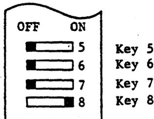
The figure at left shows the configuration for selecting Device Number 1.
