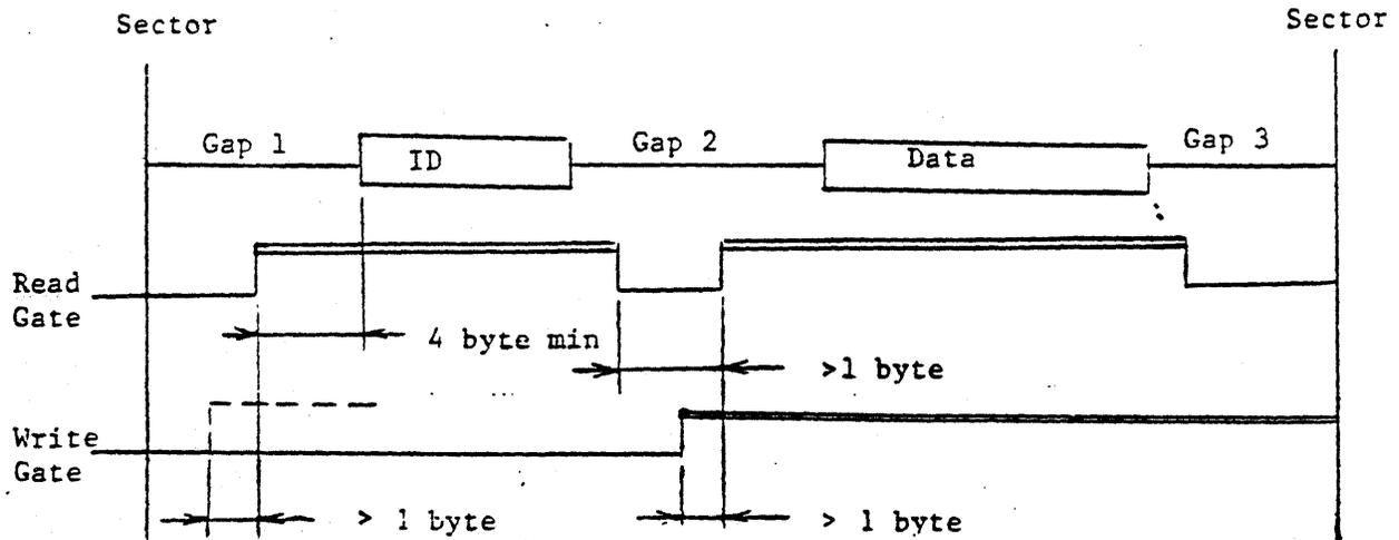
(b) The timing signals, Write Gate and Read Gate, should satisfy  $t > 1$  byte, as in the diagram, in order to avoid a write splice.
