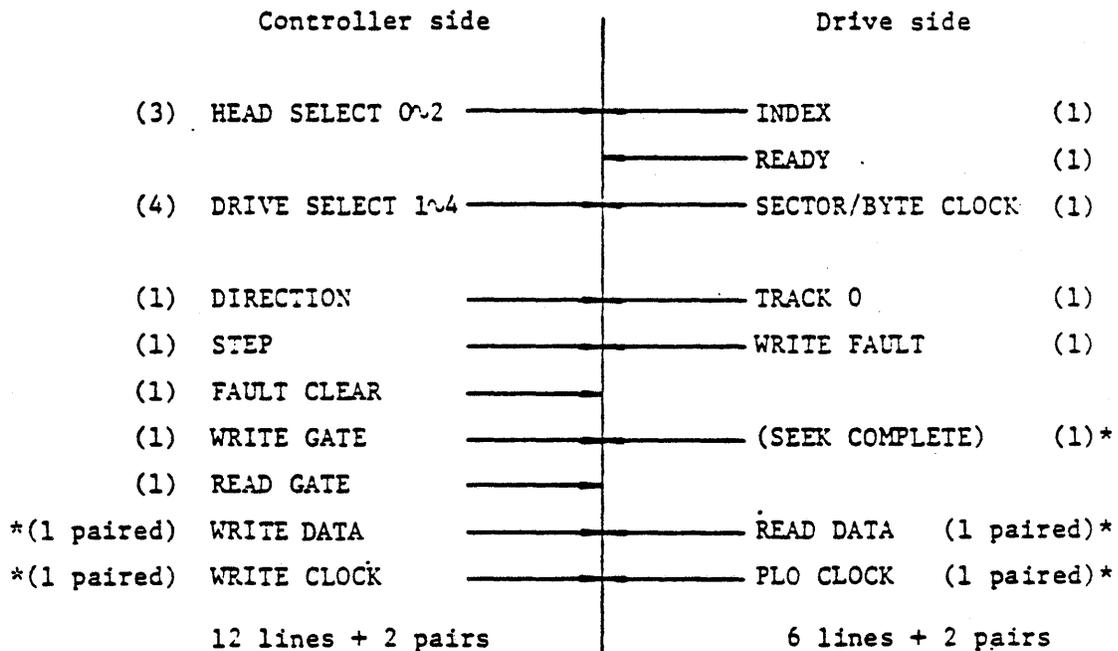
\* This signal line is connected by setting a switch on the PCB.
