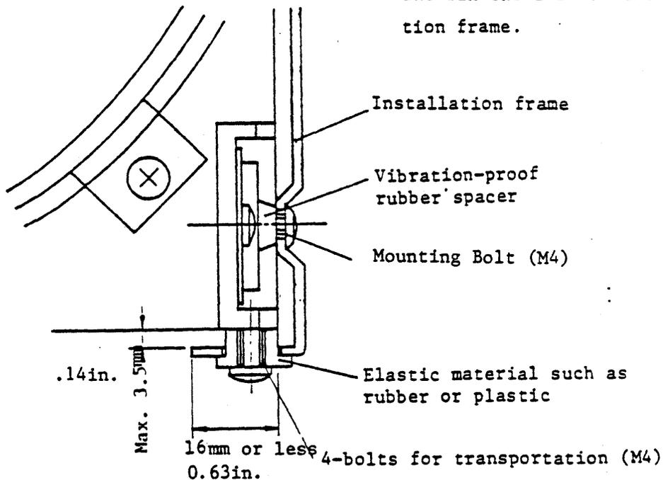
Fig. 5.4 Fixing the Unit
