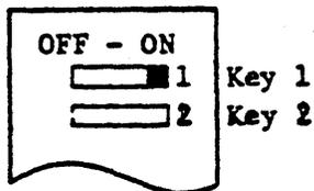
The figure at left shows the switch configuration when the INDEX/SECTOR is not sent simultaneously.
