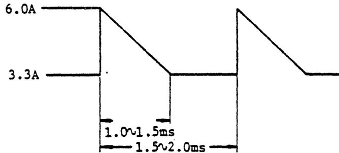
Note) The peak current (6A) in the A section flows only 3 or 4 times during one seek.
