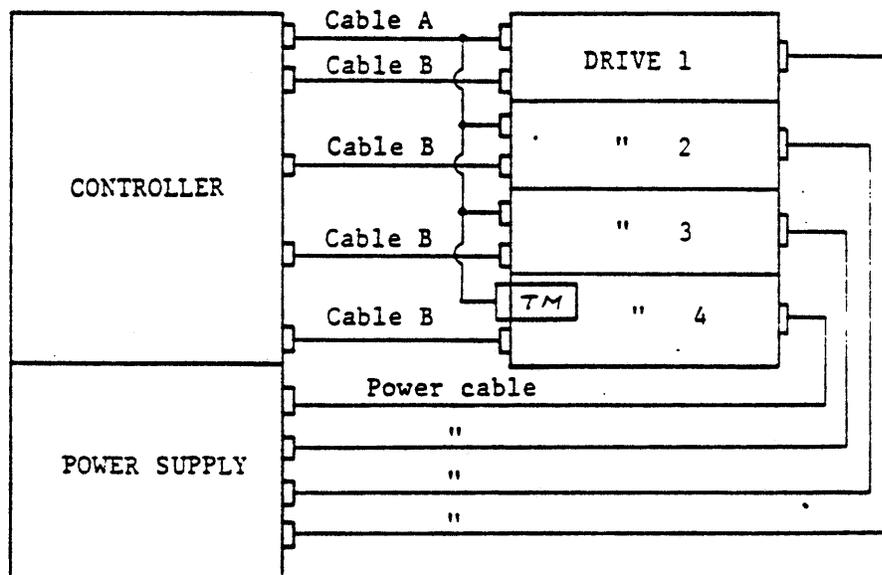
Fig. 6.3 Connecting Multiple Units
