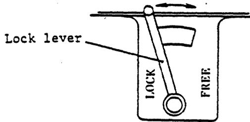
The lock is fixed (LOCK) and released (FREE) by pulling up the lever and moving it in the direction of the arrows.
