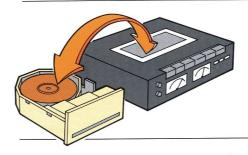
Mass Storage Back-up Video Cassette Adaptor Board provides up to 80 megabytes of formatted storage on video tape recorder.
