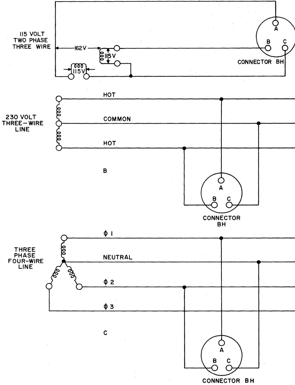
Figure 5. A-C Power Connections to Computer.
