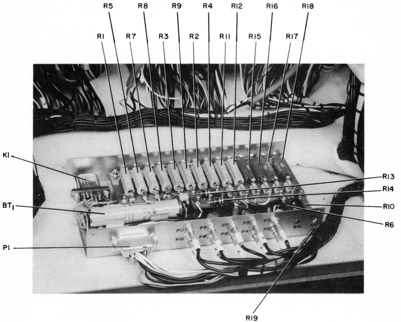
Figure 5. Reference and Check Amplifier Network 12.098.
