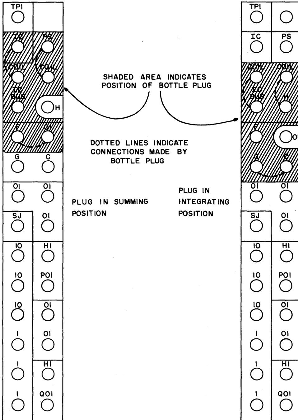
Figure 9. Combination Amplifier Patching.
