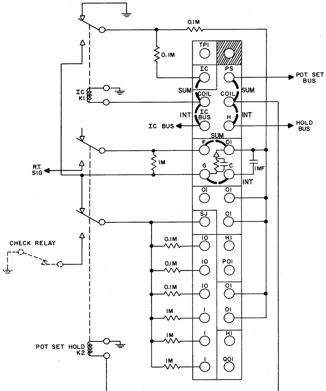
Figure 10. Combination Network Connections.
