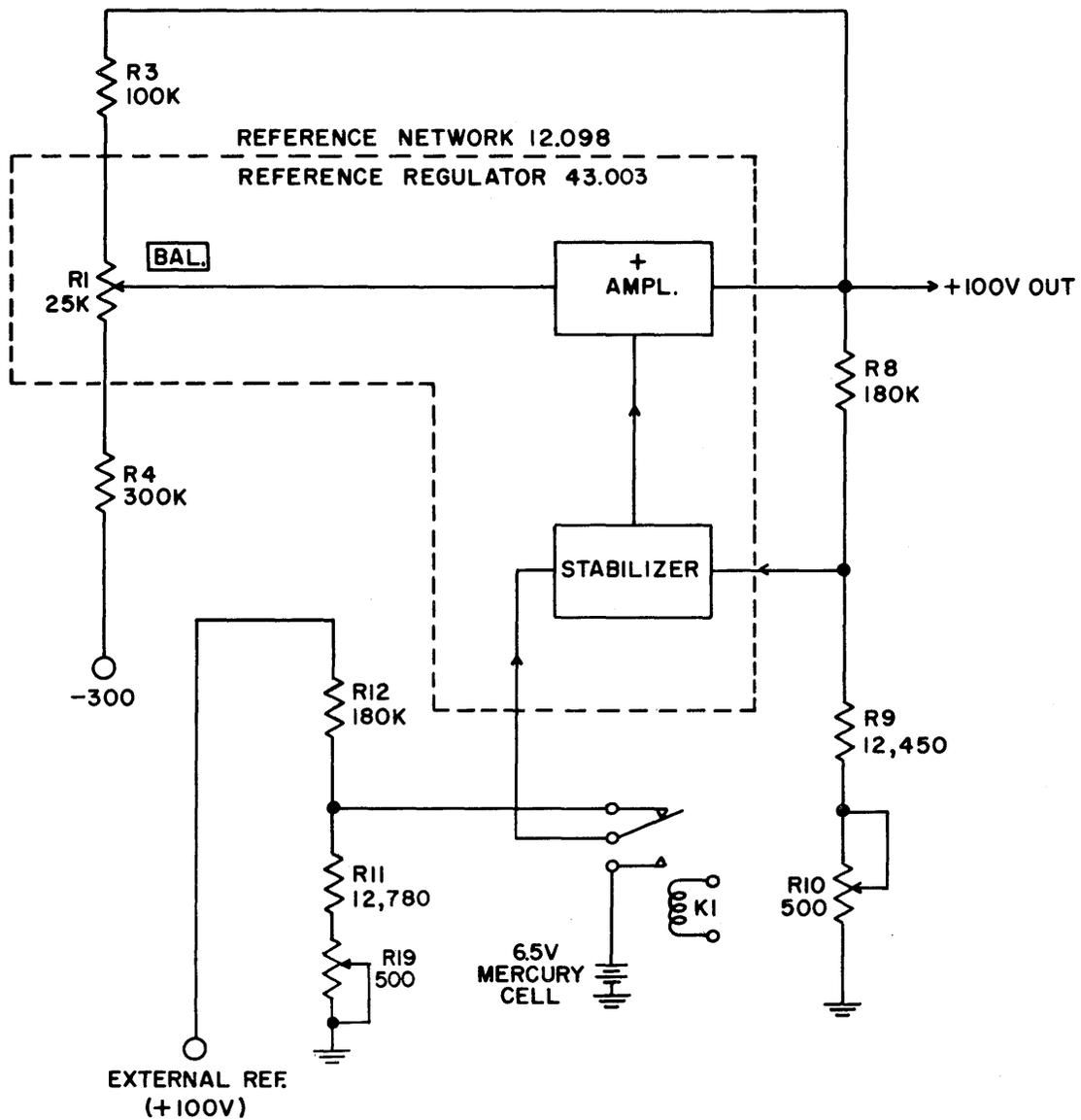
Figure 2. Block Diagram, +100 Volt Reference Source.
