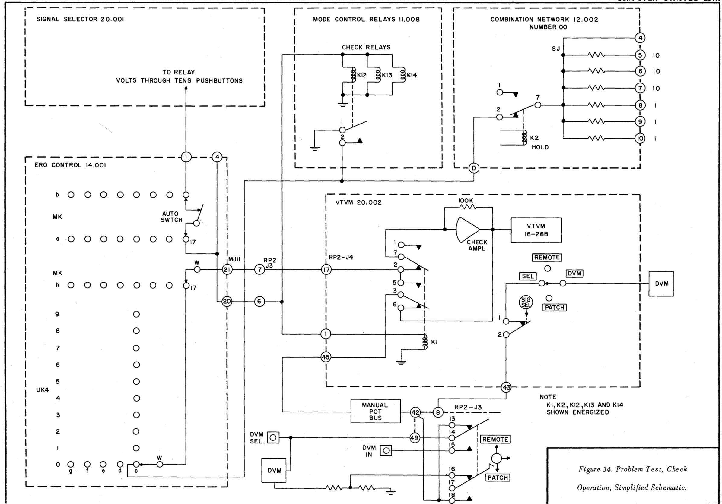
Figure 34. Problem Test, Check Operation, Simplified Schematic.
