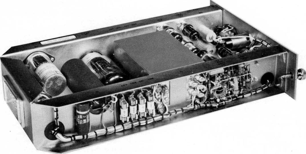
*Figure 1. Regulated Power Supply 10.017.*
