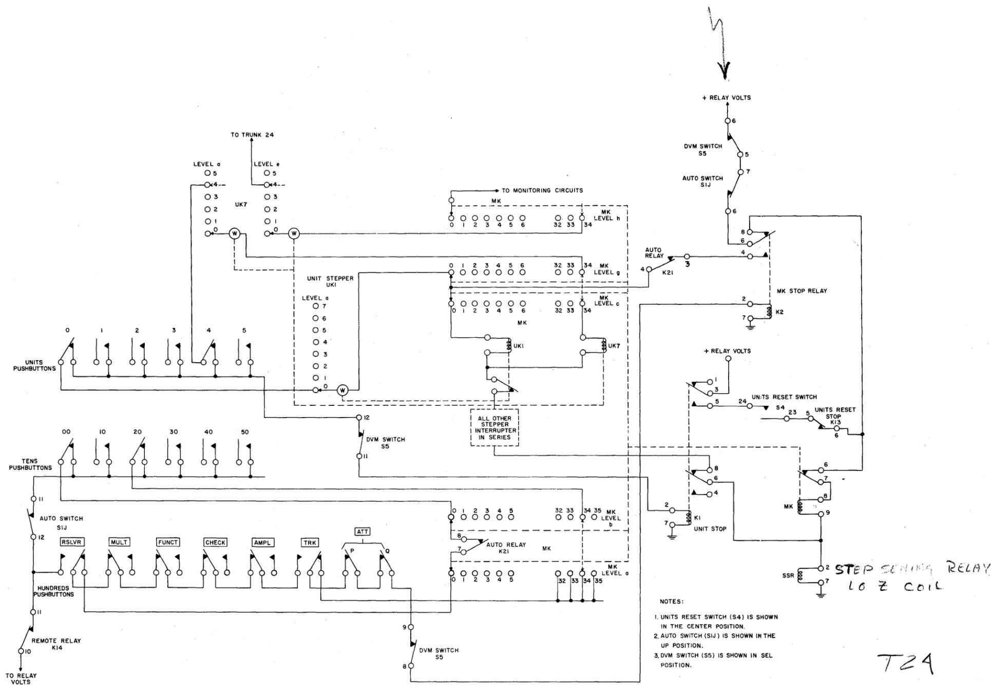
Figure 23. Manual Readout, Simplified Schematic.
