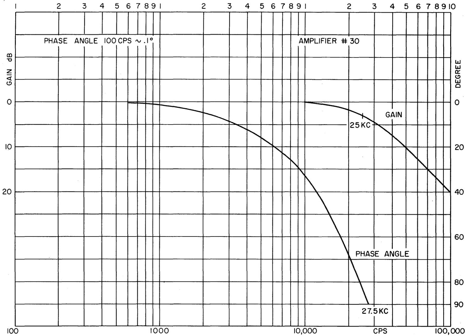
Figure 3. Amplifier High Frequency Characteristics.
