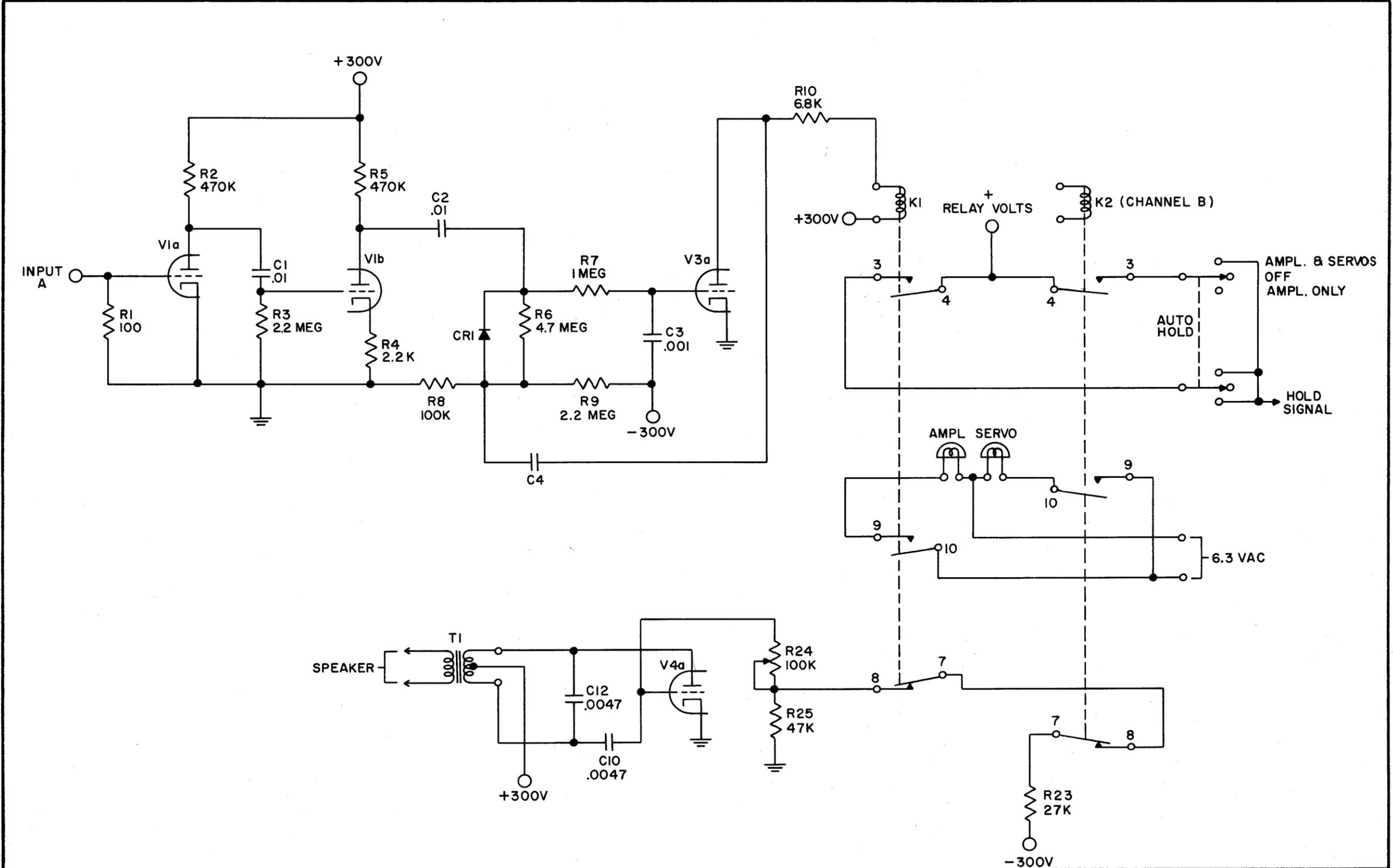
Figure 2. Dual Channel Overload Alarm,
