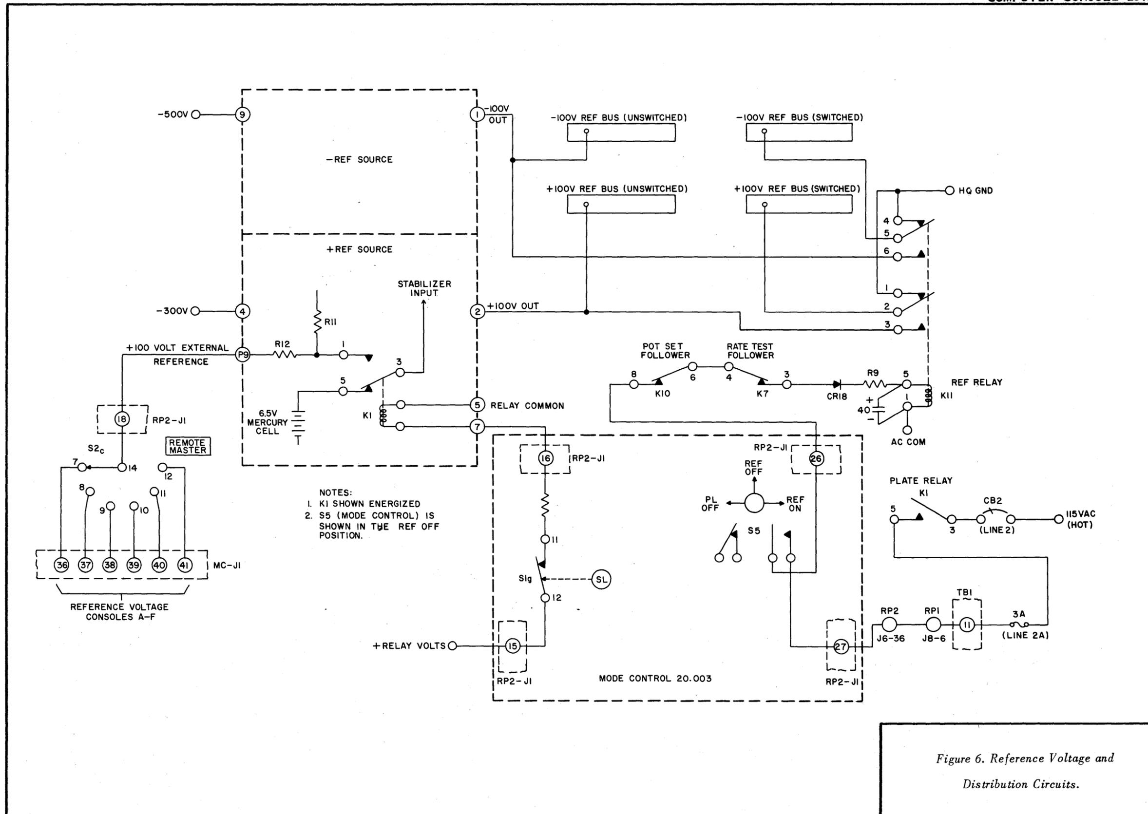
Figure 6. Reference Voltage and Distribution Circuits.
