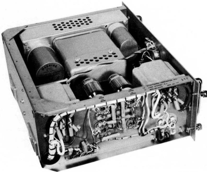
*Figure 1. Regulated Power Supply 10.001.*
