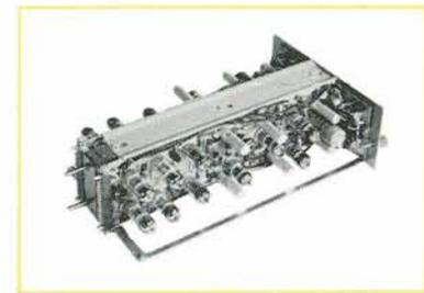
All components are plug-in, drawer type units which feature miniaturization and printed circuitry to keep maintenance to a minimum.
