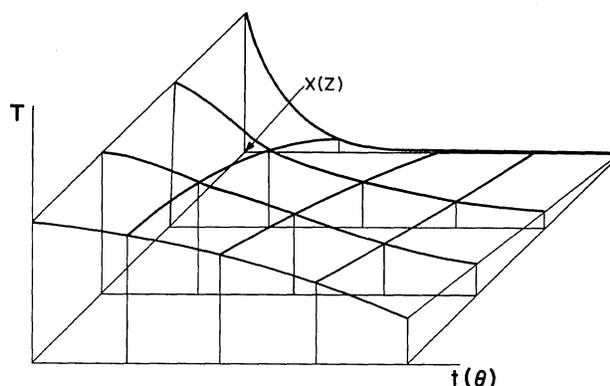
Figure 2: Sketch of Typical 3-D Plot Obtained of Temperature "Surfaces" in a Glass Slab
