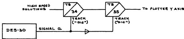
Figure 6a. Program for Fast-to-Slow Conversion (FSC)
