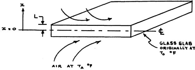
Figure 1: Glass Slab Being Air Cooled
