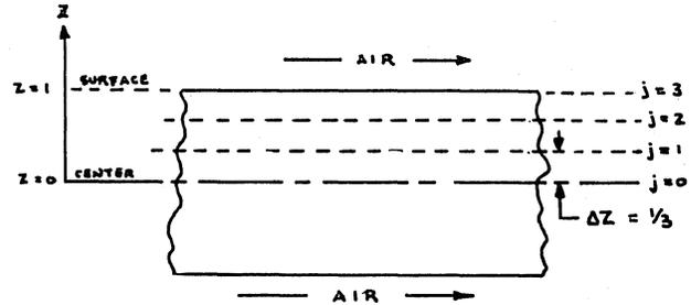
Figure 2: Definition of Points for Space Finite Differencing
