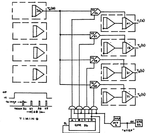
Figure 4: Program to Obtain I.C. for the Semi Serial Solution
