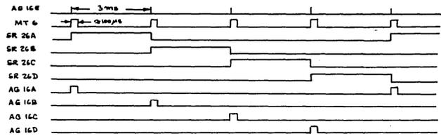
Figure 10: Timing of the Parallel-to-Serial IC Pickup Control
