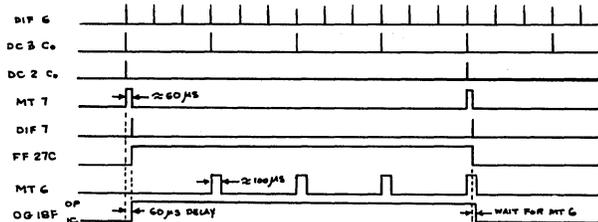
Figure 11: Master Timer Timing Diagram
