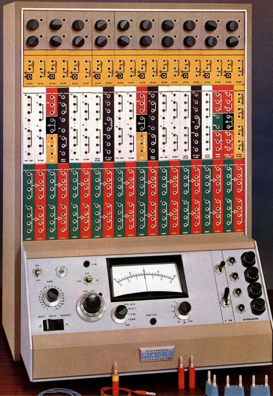
New EAI computer puts the advantages of analog computation right at your desk. Accurate to 0.1%, it is capable of performing the mathematical operations required in the solution of 95% of your routine engineering problems. Differential equations, basic to most engineering problems, can now be solved with surprising rapidity. Even if you have never seen a computer before, you can learn to operate the TR-10 as easily as you learned to use a slide rule.
