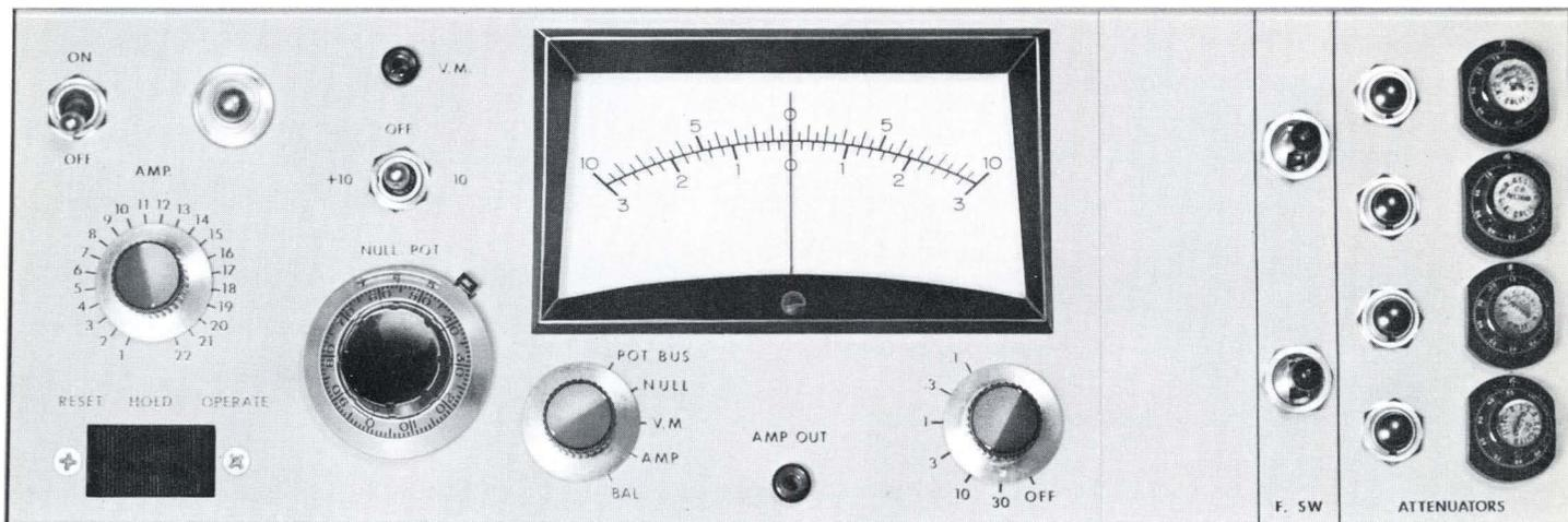
**CONTROL PANEL** has been designed for ease of operation. All knobs, buttons and switches are clearly marked and entire panel is inclined to make elements easier to see and reach. Human engineered control panel is employed in setting coefficient potentiometers, reading out problem variables, controlling computer operating mode (i.e.—hold—operate—reset), controlling primary power to computer and periodic manual balancing of operational amplifiers.
