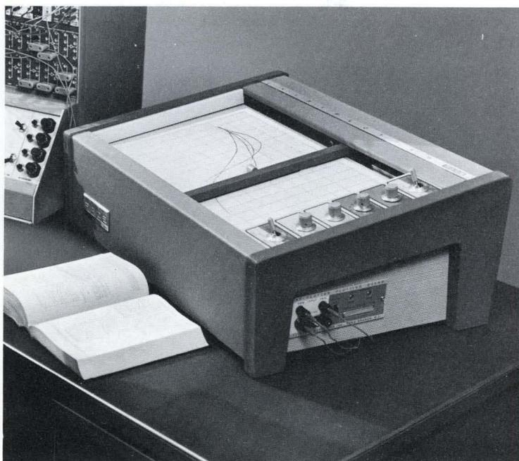
**X-Y PLOTTER** — Model 1100E Variplotter provides highly accurate recording of any two problem variables. Re-runs can be easily made with different parameter values for comparison studies. The plotter may also be used as a time-based recorder or function generator. Write for further details.
