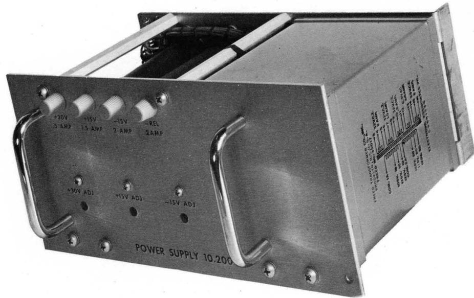
FIGURE 3.1-1. REGULATED POWER SUPPLY 10.200
