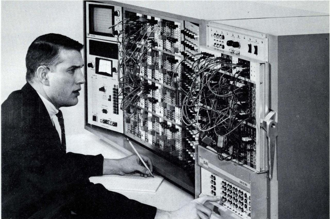
The DES-30 (Digital Expansion System) is a general-purpose, low-cost digital logic system. Though capable of operating autonomously, it was primarily designed as an expansion to the PACE® TR-48 Analog Computer — providing basic
