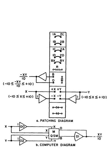
Figure 2. Multiplication-Patching and Computer Diagrams
