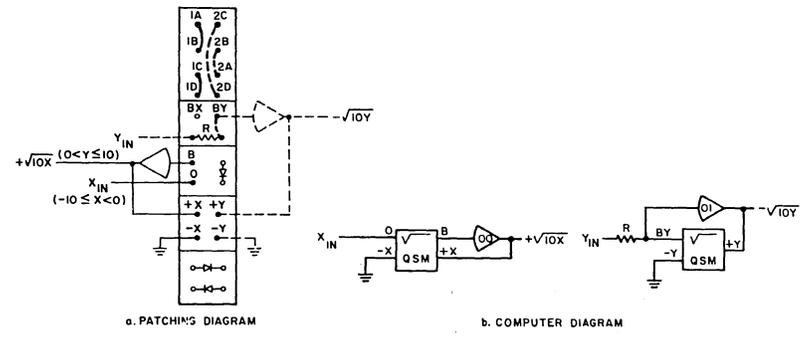
Figure 5. Square Root Extraction-Patching and Computer Diagrams
