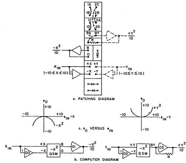
Figure 3.  $X^2$  Squaring-Patching and Computer Diagrams
