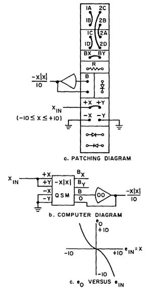
Figure 4.  $X|X|$  Squaring-Patching and Computer Diagrams
