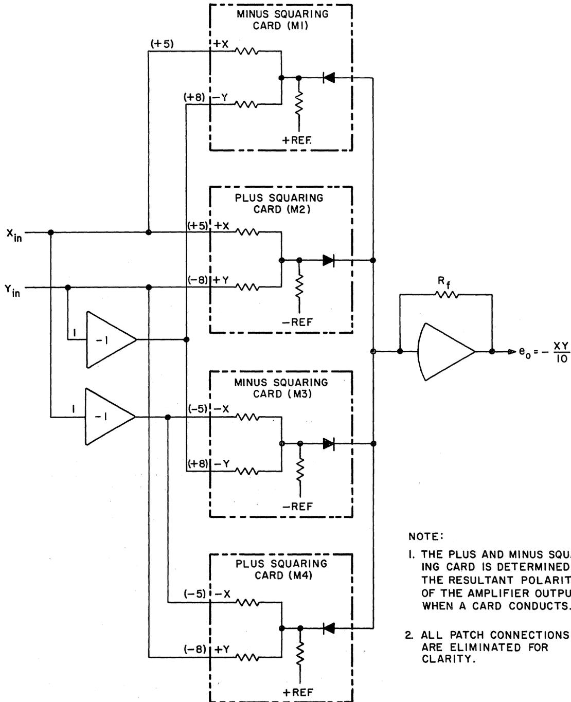
Figure 12. Four Quadrant Quarter-Square Multiplier, Simplified Schematic
