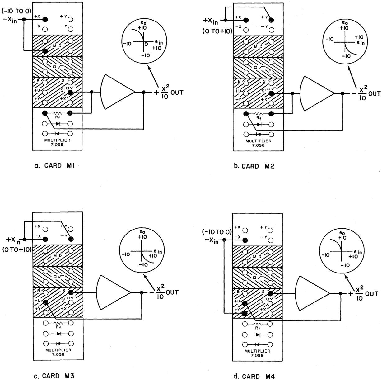
Figure 18. Patching for Individual Card Testing
