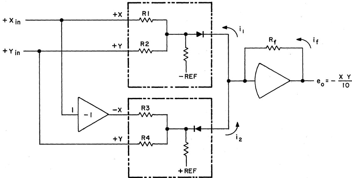
Figure 11. Two-Network Quarter-Square Multiplier, Simplified Schematic
