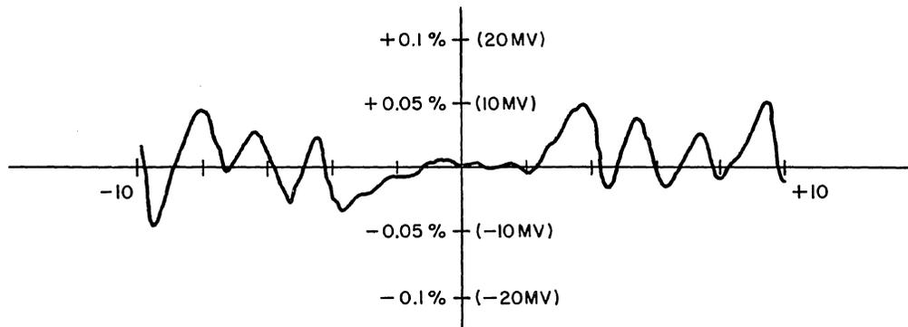
a. TYPICAL ERROR CURVE FOR Y = +RAMP, X = +6.65 VOLTS
