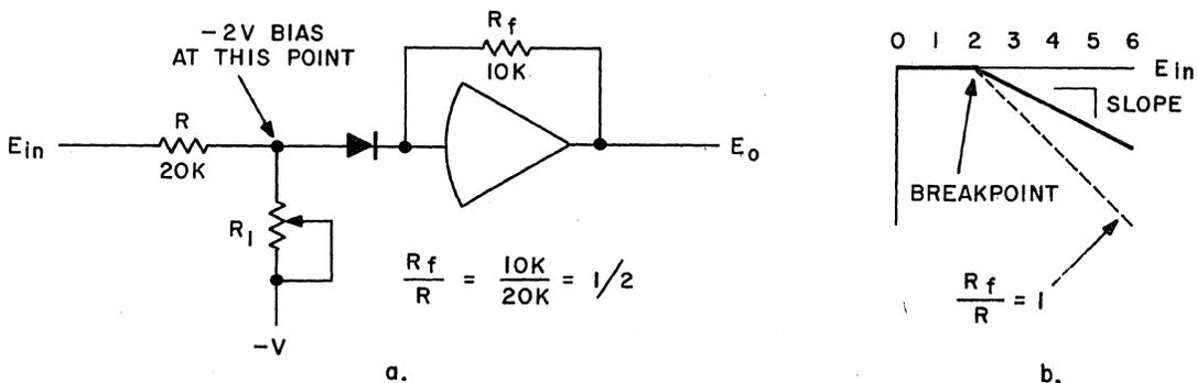
Figure 8. Simple Diode Function Generator
