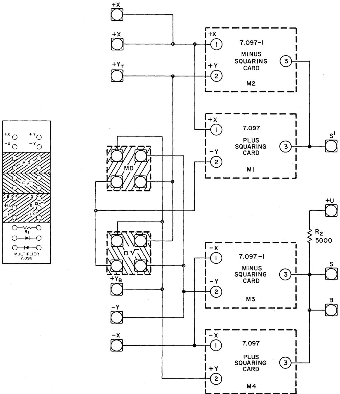
Figure 2. Patching Block and Simplified Schematic
