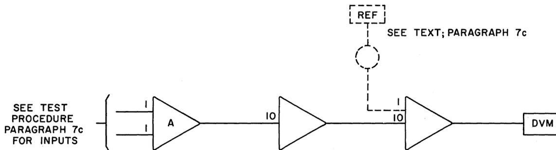
a. RESISTOR MATCHING TEST SETUP
