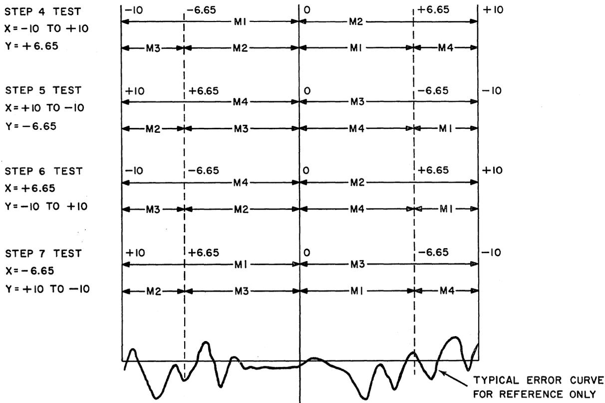
Figure 17. Error-Test Card Operation Sequence
