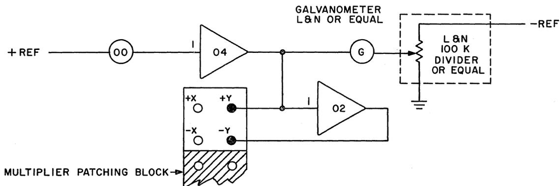
b. ATTENUATOR 00 ADJUSTMENT SETUP
