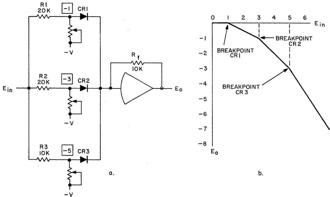
Figure 9. Three-Network Diode Function Generator
