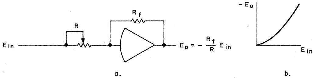
Figure 7. Elementary Function Generator
