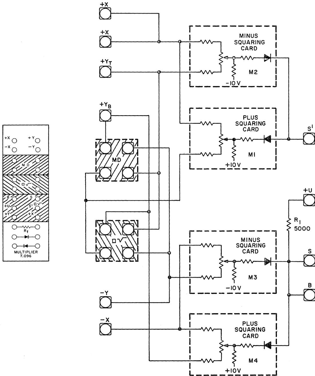
Figure 19. Quarter-Square Multiplier, Simplified Schematic and Patching Block
