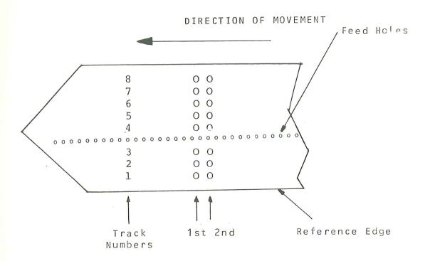
With the tape oriented as shown and the observer looking down on to the tape, the direction of forward tape movement is from right to left, and the first character of date (the most significant character as entered from a tapewriter-like device) is the one farthest to the left (1st). The next most significant character follows it (2nd) etc.
