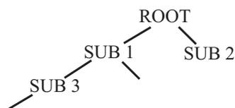
The hierarchy shall consist of a number of levels (i.e. for n levels: level 1, level 2, ..., level n). The Root Directory shall be the only directory at level 1 of the hierarchy.
