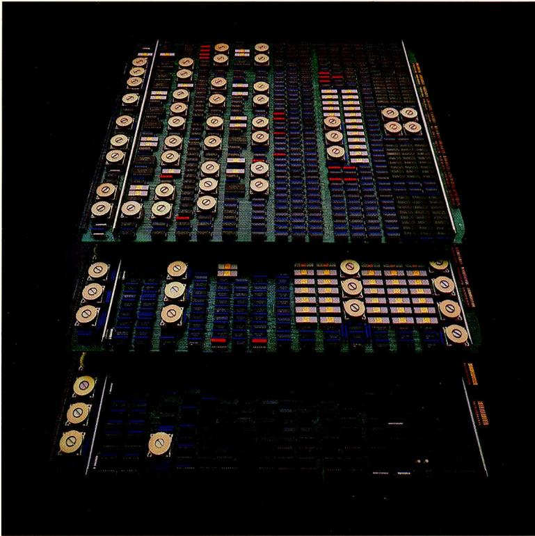
High-density packaging of ELXSI Processor and Service Processor boards, using ECL/LSI Components.
