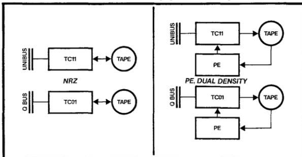
Thus for the PDP-11 Unibus series of DEC computers, Emulex offers a single controller that will handle tape transports having the following ranges:
