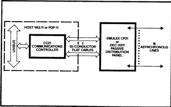
The CC21 is packaged on a single hex height 2-sided pcb. The unit occupies a single SPC slot, presents one bus load, and draws approximately 8 amps of power from +5 volts, and 0.25 amps of power from +15 volts.
