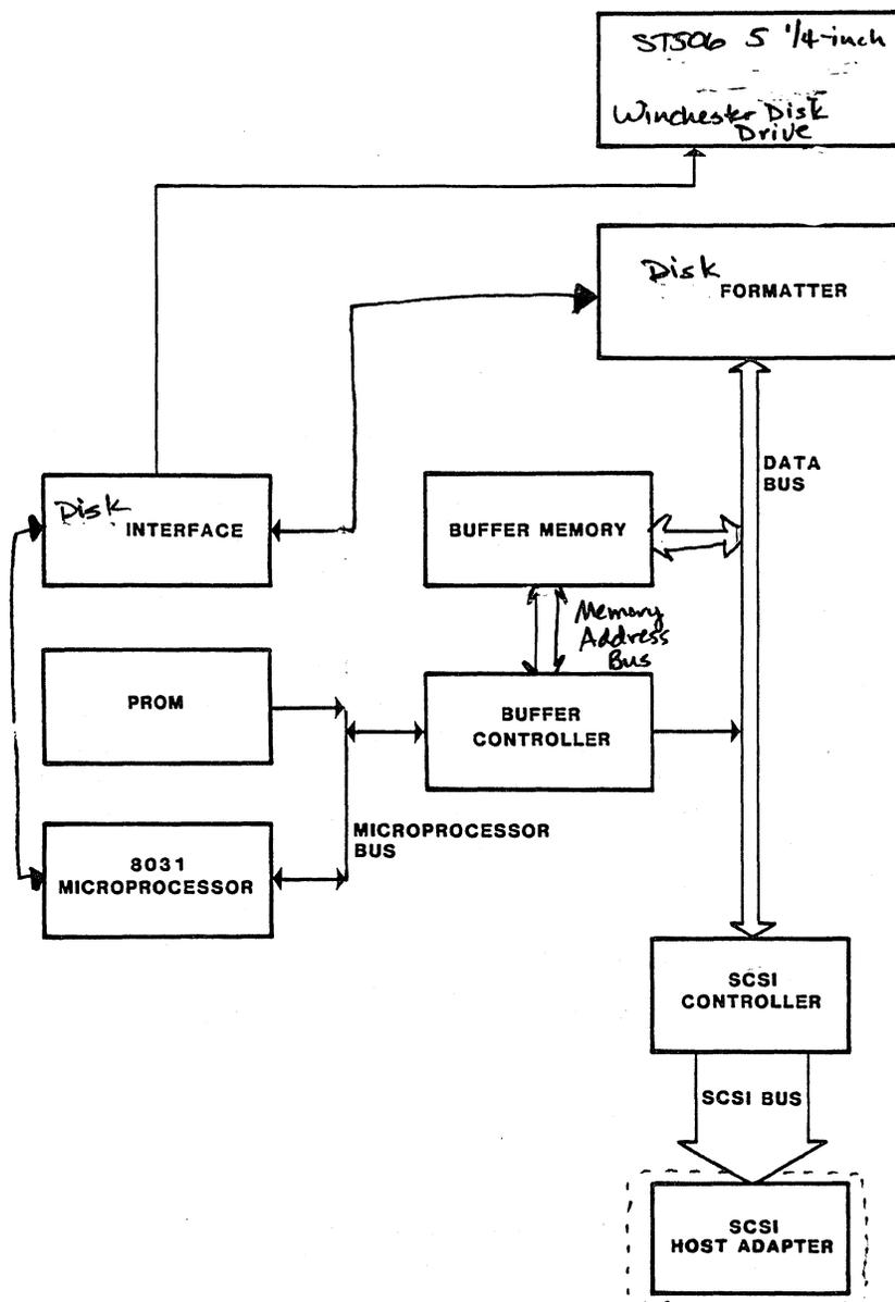
Figure 5-1. MD01 SCSI Controller Block Diagram
