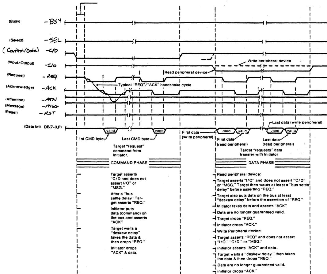
Figure 6-3. SCSI Bus Timing Diagram (Sheet 2 of 3)
