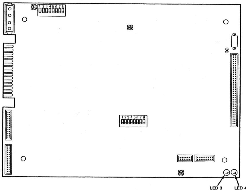
Figure 4-1. Location of LEDs on MD01 Controller
