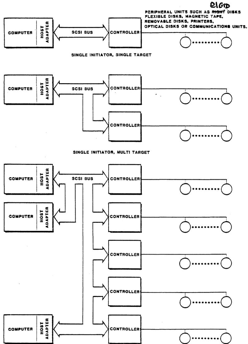
Figure 7-1. Sample SCSI Bus Configurations
