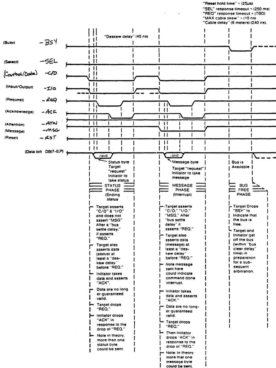
Figure 6-3. SCSI Bus Timing Diagram (Sheet 3 of 3)
