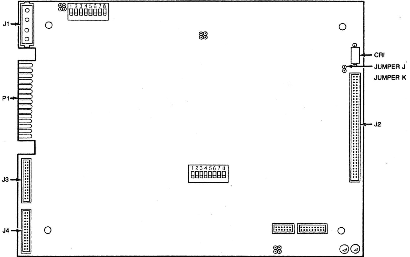
Figure 3-1. MD01 Switch and Jumper Locations
