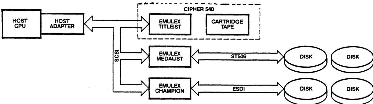
Figure 1-2. Sample SCSI Bus System Configuration
