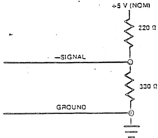
Figure 6-2. SCSI Bus Signals Termination
