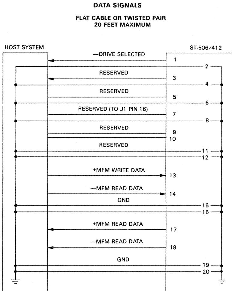
Figure 6-5. Data Pin/Signal Assignments at Disk Drive Interface
