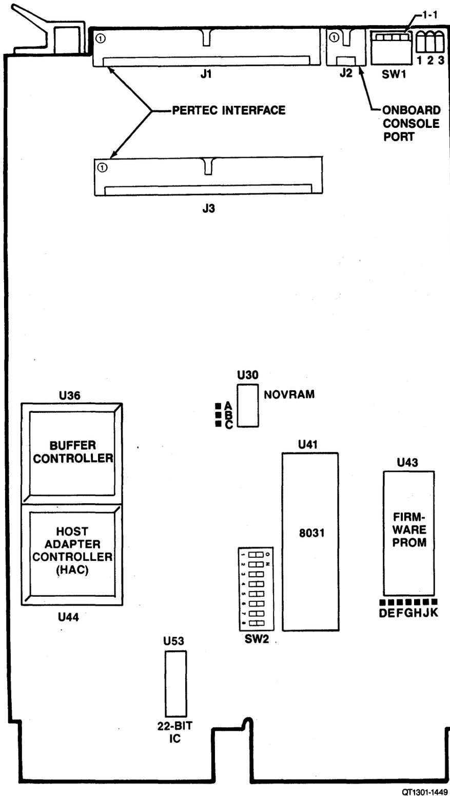
Figure 2-3. QT13 Tape Coupler Assembly
