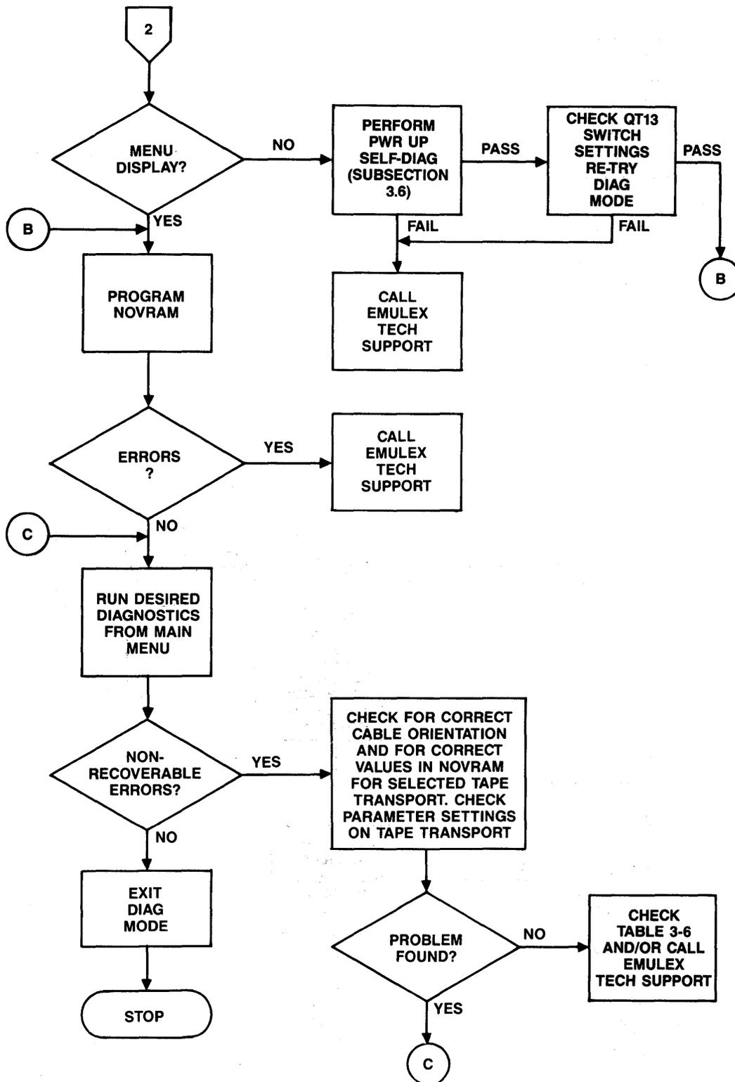
Figure 3-2. Fault Isolation Flow Chart (Sheet 2 of 2)
