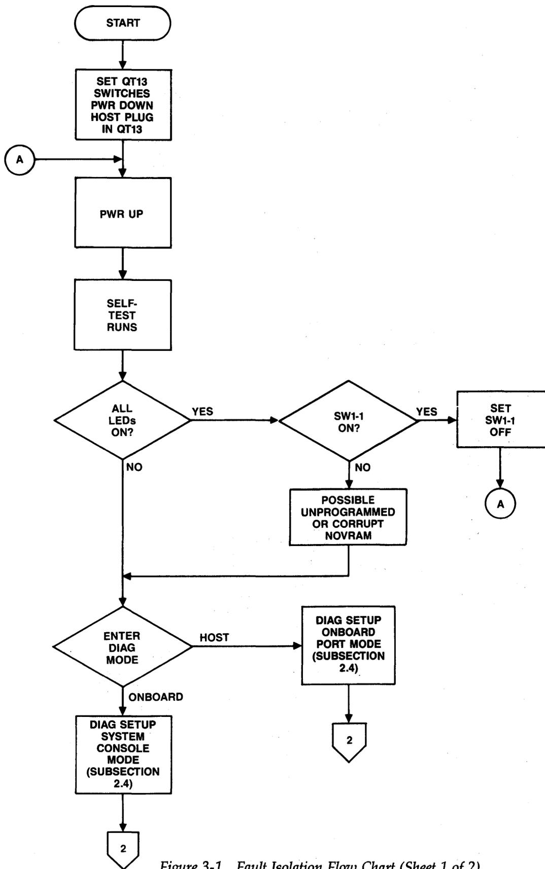
Figure 3-1. Fault Isolation Flow Chart (Sheet 1 of 2)
