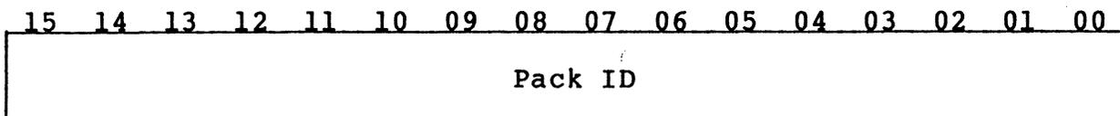
During Write Header commands the MPR is loaded with the Pack ID that is used for the Bad Sector File. The MPR must be loaded prior to the issuance of the Write Header Command.
