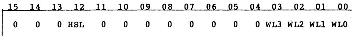
The figure above defines the bits of the MPR during a Multipurpose Command. The bits should be set in this register prior to issuing the Multipurpose command.
