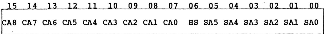
For a read or write operation, the DA register is loaded with the address of the first sector to be transferred. As each successive sector is transferred, the DA register is automatically incremented.
