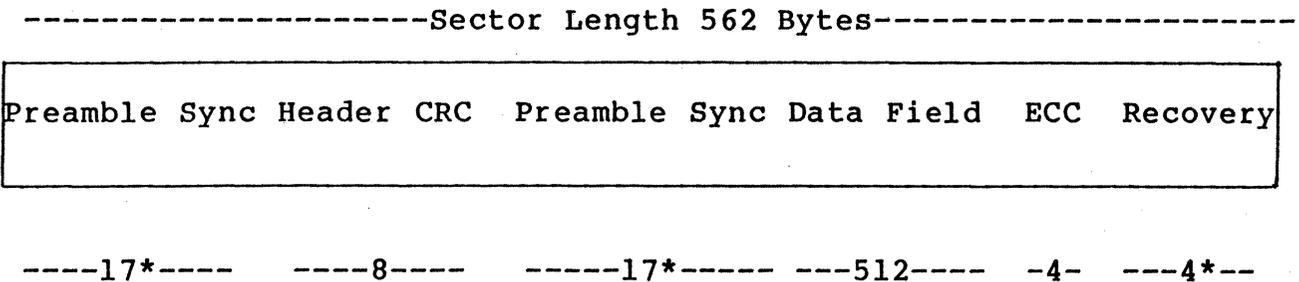
\*Values shown are minimums which apply to most Winchester type units. However, these values may vary to accomodate different physical drive types and are determined by configuration PROM data.
