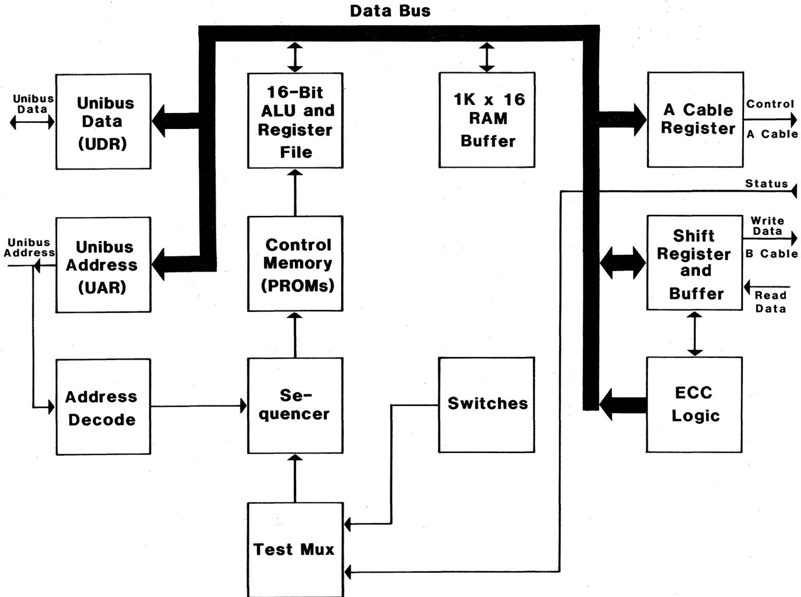
**Figure 2-1 SC21 Block Diagram**
