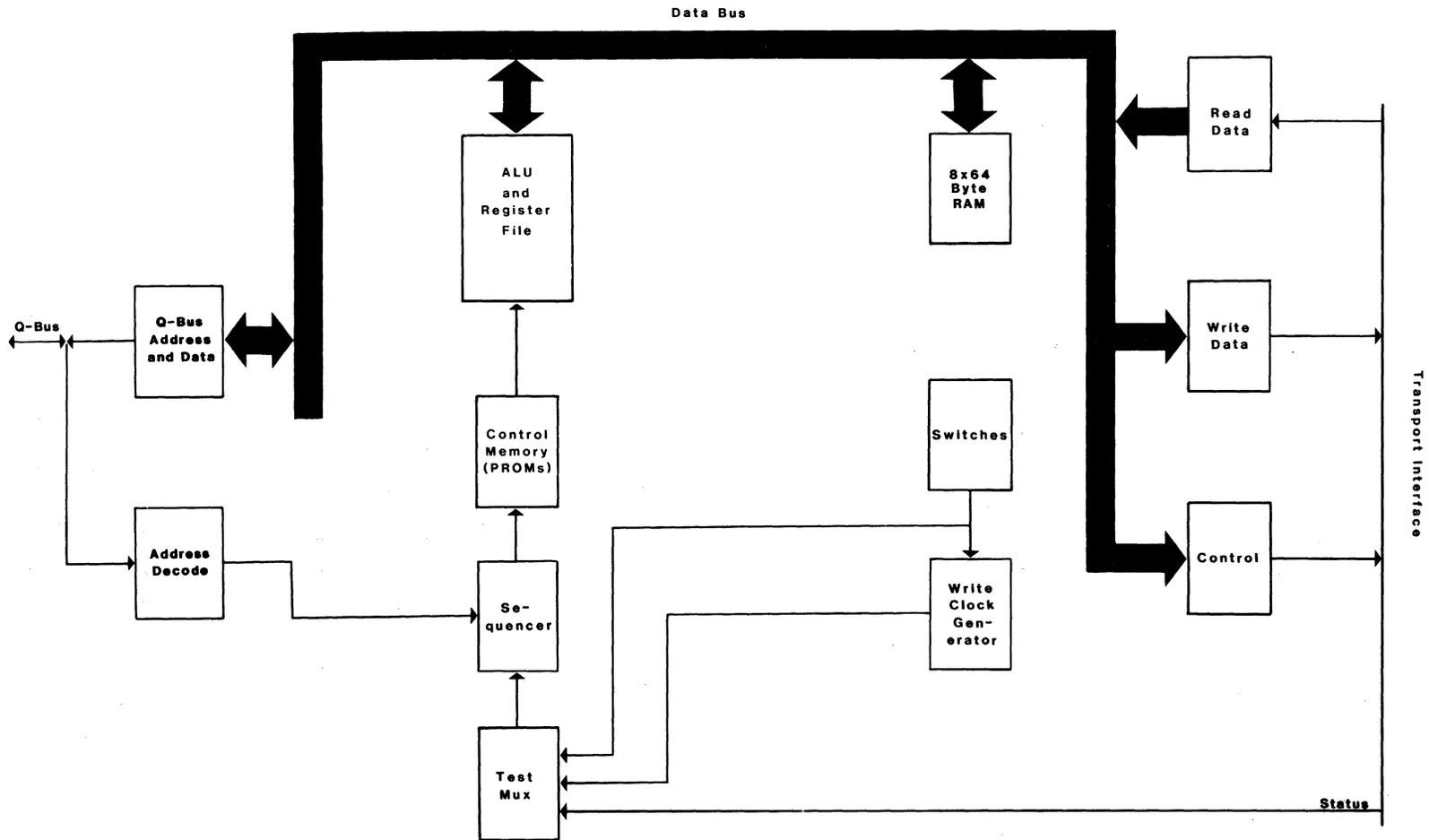
Figure 2-2 TC02 Block Diagram
