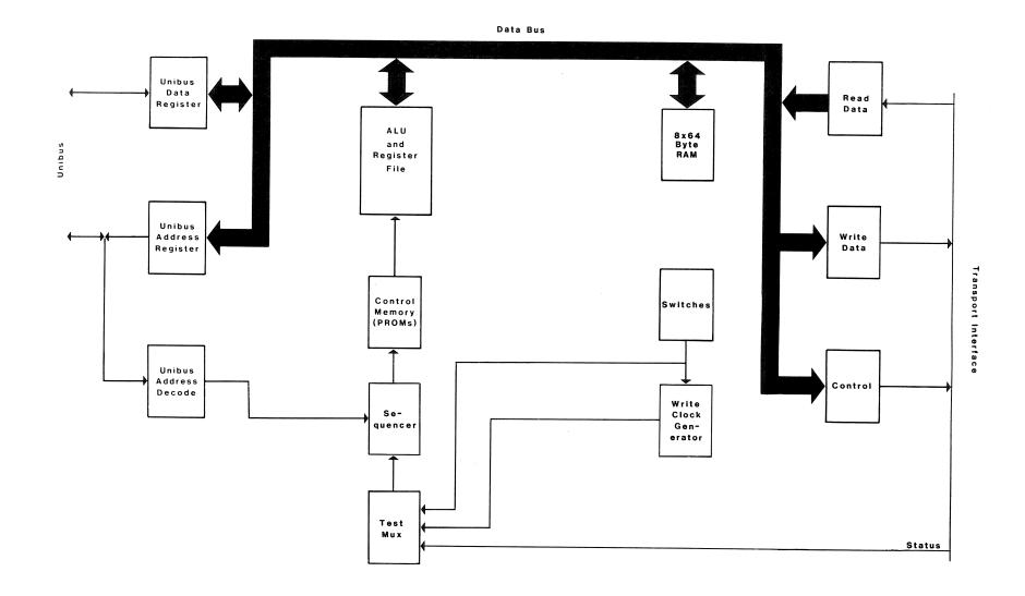
Figure 2-2 TC12 Block Diagram
