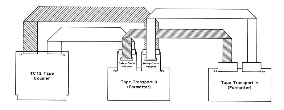
Figure 4-3 Tape Transport Cabling
