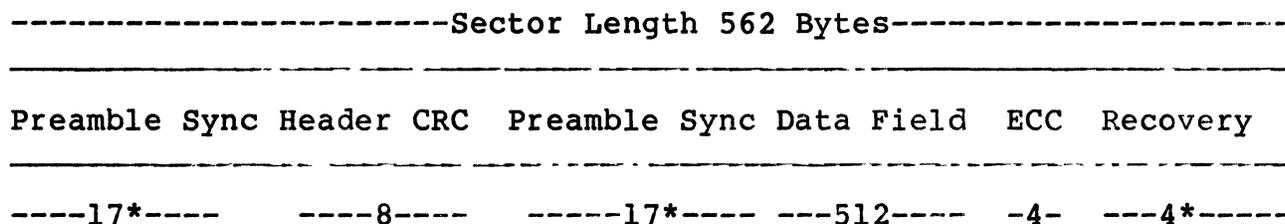
\*Values shown are minimums which apply to most Winchester-type units; however, these values may vary to accommodate different physical drive types and are determined by configuration PROM data.
