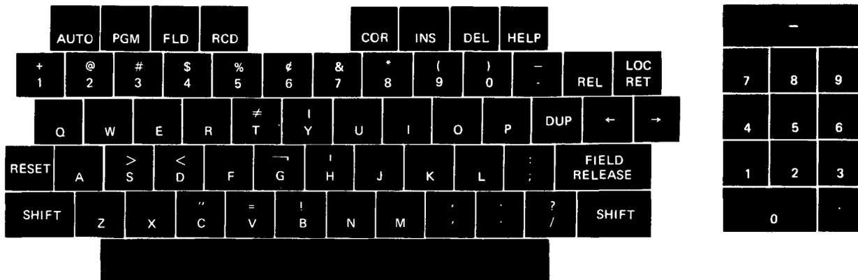
Figure 2-2 System 480 Typewriter Keyboard
