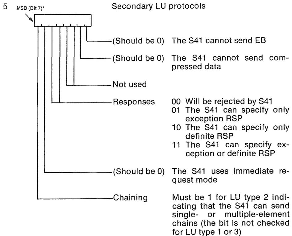
\*Note: IBM designates the most significant bit (Bit No. 7) as bit No. 0.
