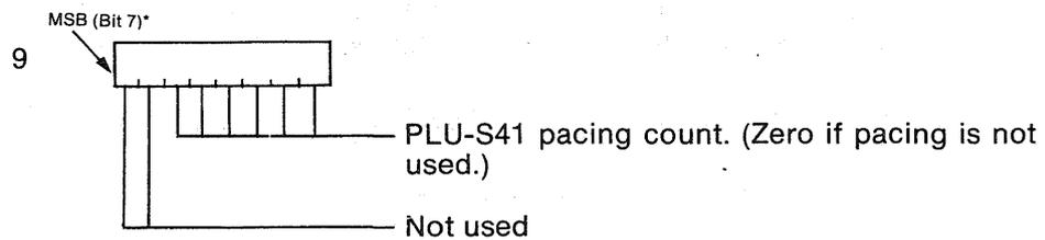
\*Note: IBM designates the most significant bit (Bit No. 7) as bit No. 0.
