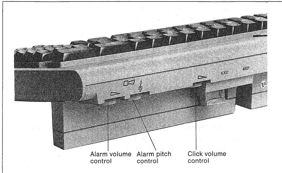
Fig. 4. Keyboard controls
