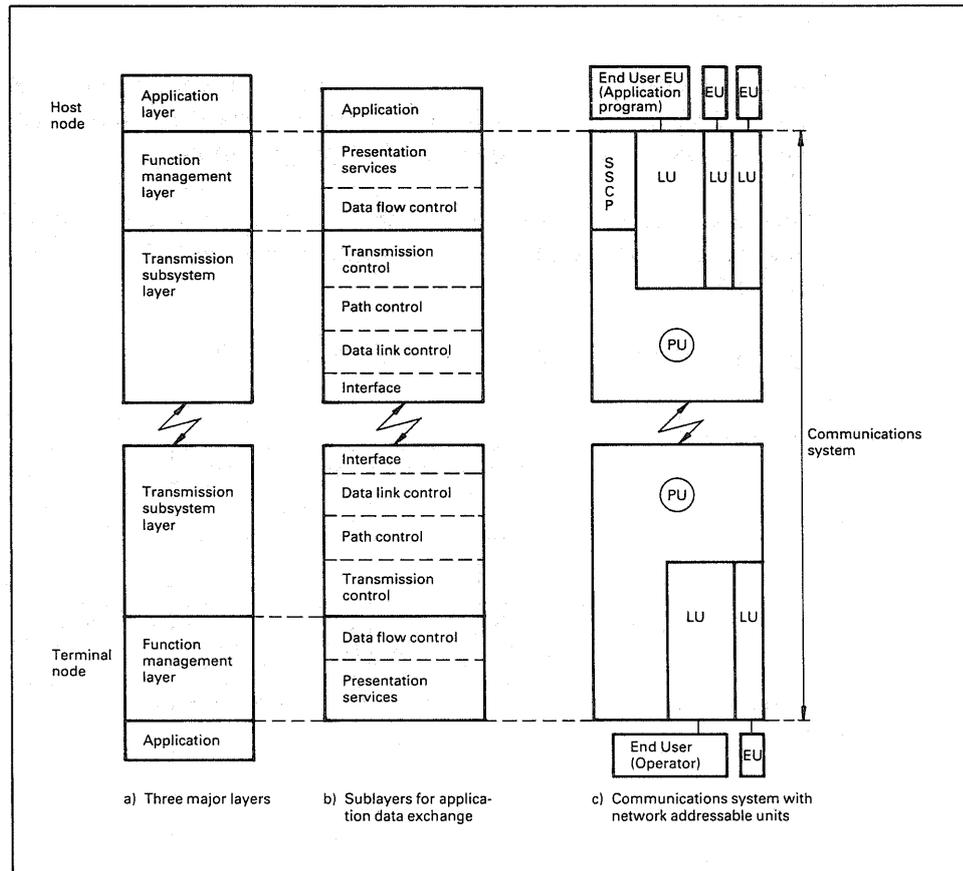
Fig. 1. SNA layering arrangement
