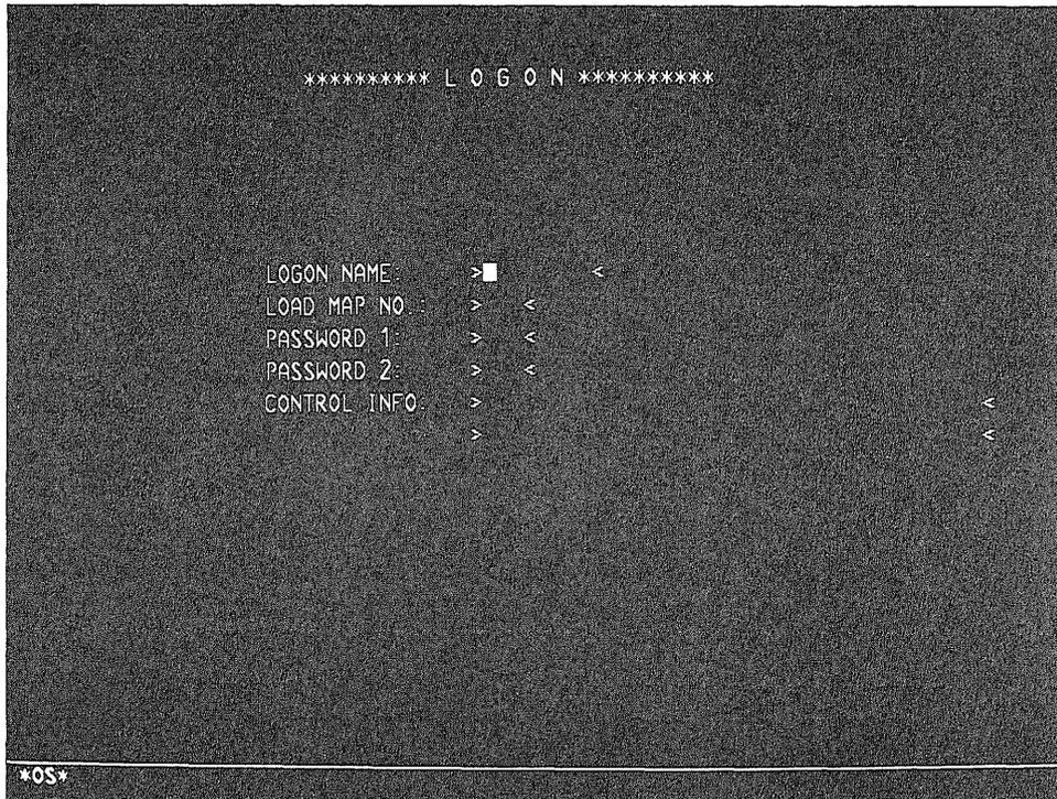
The operator then enters the desired name (em 3274 for example), the load map number (001 for example) and, if required, other items of information. The ENTER key shall then be depressed. When the logon operation is completed, the menu will disappear and be replaced by an empty screen or another form, depending upon which software has been loaded. \*OS\* will still appear on the message line unless the emulation software has been loaded, in which case \*EM\* will appear on the message line.
