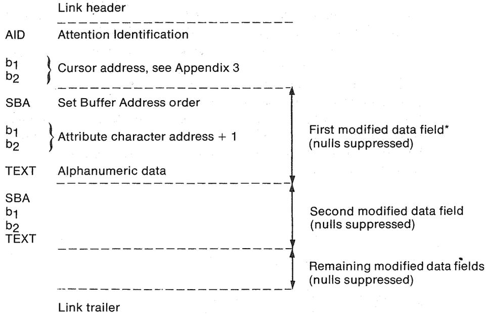
\* Note: The SBA order and attribute character address + 1 are not obtained for an unformatted screen. Instead, all text in the buffer (nulls suppressed) follows the cursor address.
