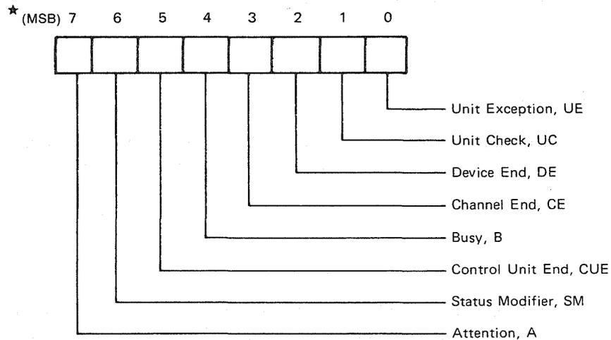
★ Note: IBM designates the most significant bit (MSB) as No. 0
