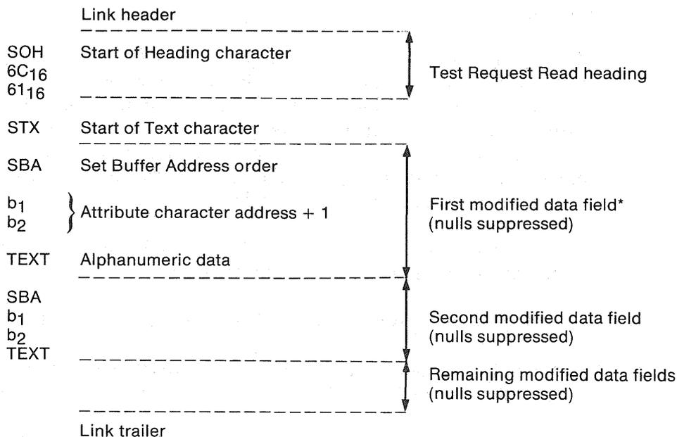
\* Note: For an unformatted screen the SBA order and attribute character address + 1 are not obtained. Instead, all text in the buffer (nulls suppressed) follows STX.
