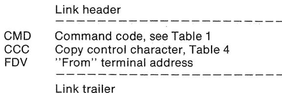
*Fig. 7. Copy command, message layout*
