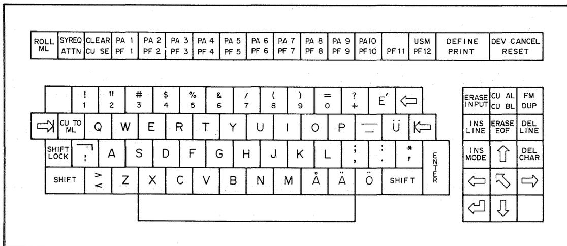
**Keyboard Layout for Swedish/Finnish Data Entry Keyboard Unit**
