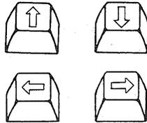
Moves the cursor one character position in the direction indicated by the arrow on the key. The cursor may be moved into any character location, including unprotected and protected numeric and alphanumeric character and attribute character locations, through the use of these keys.
