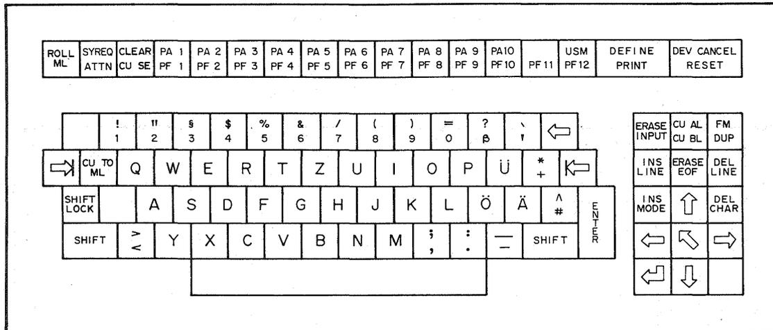
**Keyboard Layout for Austrian/German Alternate Typewriter Keyboard Unit**
