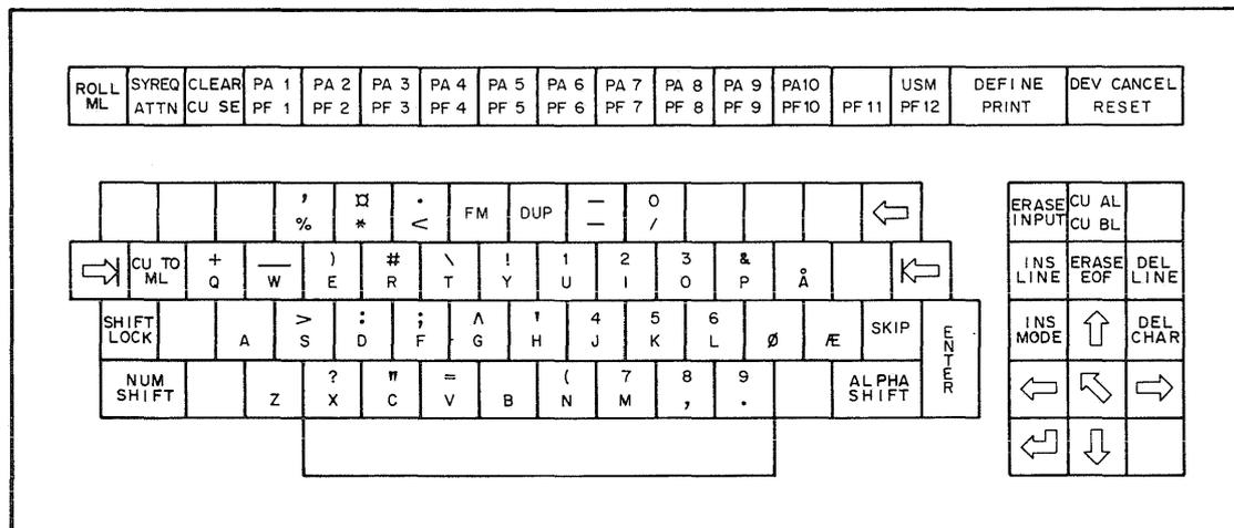
**Keyboard Layout for Austrian/German Typewriter Keyboard Unit**
