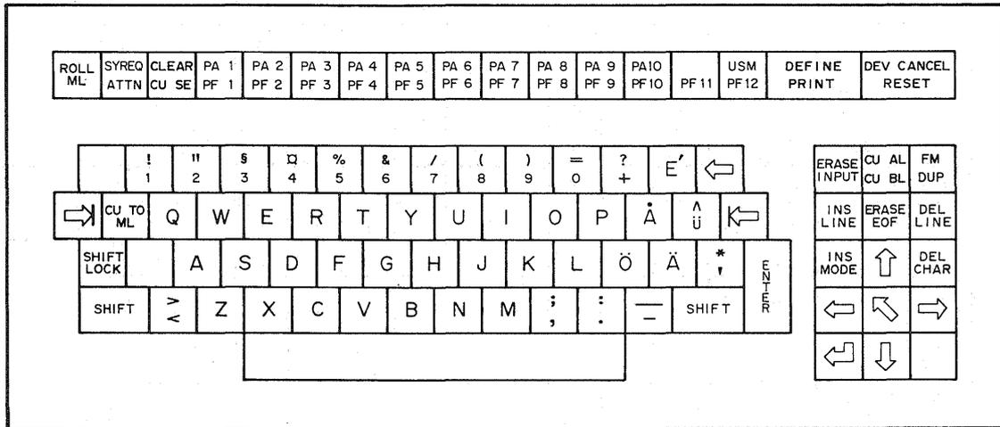
**Keyboard Layout for Swedish/Finnish Alternate Typewriter Keyboard Unit**
