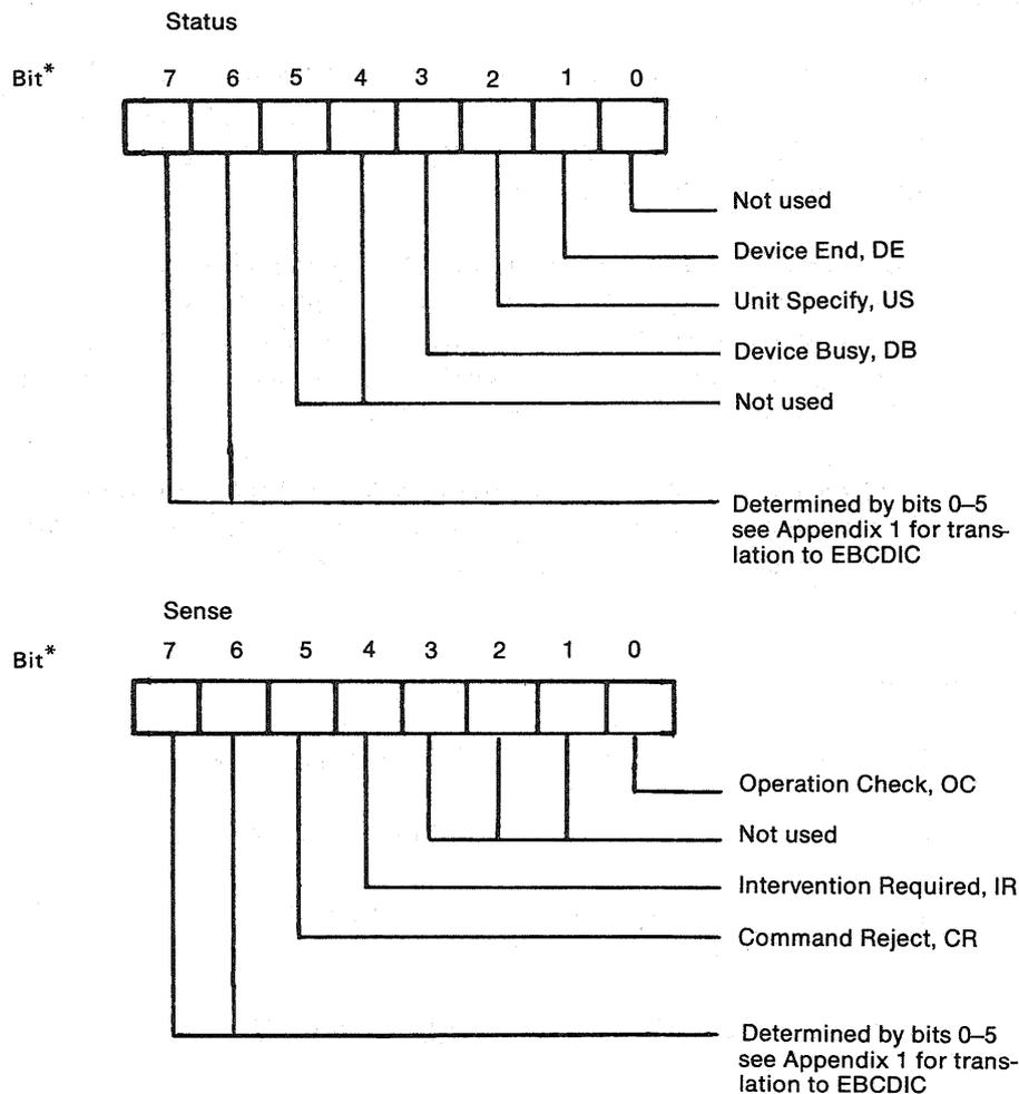
\*Note: IBM designates the most significant bit (bit No. 7) as No. 0.
