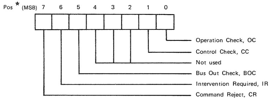
\* Note: IBM designates the most significant bit (MSB) as No. 0
