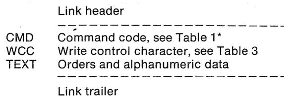
\* Note: In local operation, the command code is included in the link header and distributed via the CCW.
