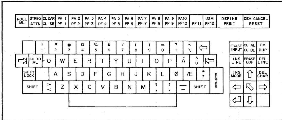
**Keyboard Layout for Danish/Norwegian Alternate Typewriter Keyboard Unit**
