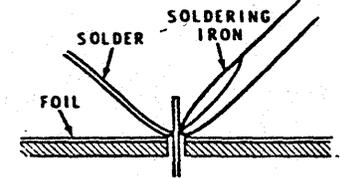
3. As the solder begins to melt, allow it to flow around the connection. Then remove the solder and the iron and let the connection cool.
