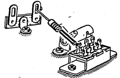
NOTE: Use sleeving when it is called for to provide insulation.
