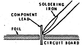
2. Then apply solder to the other side of the connection. IMPORTANT: Let the heated lead and the circuit board foil melt the solder.
