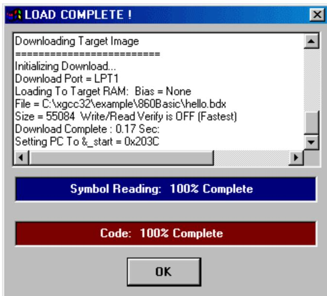
Figure 2.3: Downloading the BDX file to the target
