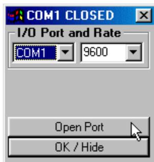
*Figure 2.4: Select the appropriate COM port for your PC and set it to 9600 baud.*
