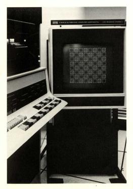
The LDS-1 operates as an independent stored program processor, sharing memory with the PDP-10. In its complete form, the system contains all the high-speed digital arithmetic logic required to rotate, translate, window, and—in three dimensional operation—to place into perspective, the objects defined by the display program.
