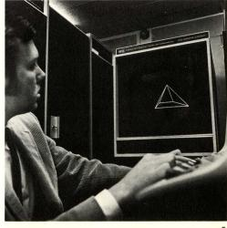
Operating the LDS-1 display is only one of the tasks that the PDP-10 can perform. At the same time that the display is in operation, graphics and other programs can be developed on-line by as many as 63 simultaneous users; batch processing can be performed for multiple program streams, or the system can handle other real-time tasks.
