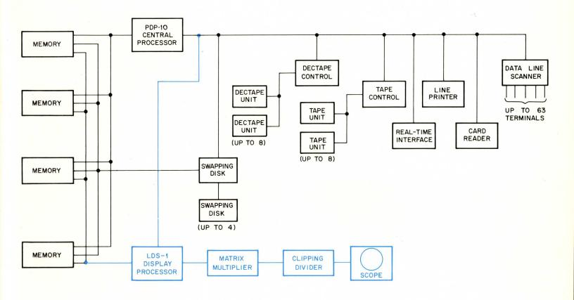
The LDS-1 display system and the PDP-10 general-purpose computer combine to form an extremely powerful and versatile system for interactive graphics and computer-aided simulation. At the same time, the combined system provides extensive facilities for terminal time-sharing, batch processing, and real-time data acquisition and analysis.
