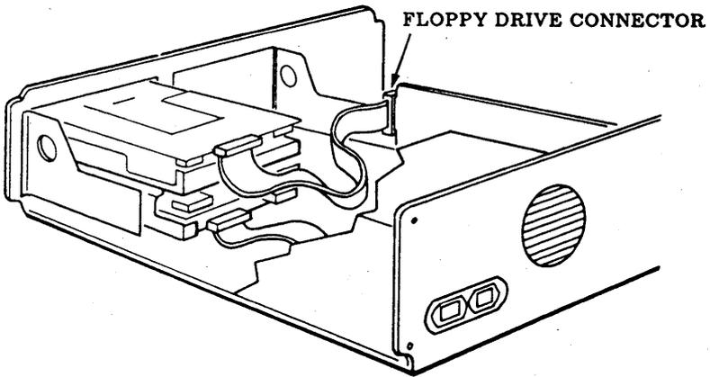
**Figure 26: Connecting the Floppy Controller Cable to the Combination Tape/Floppy Controller Card**
