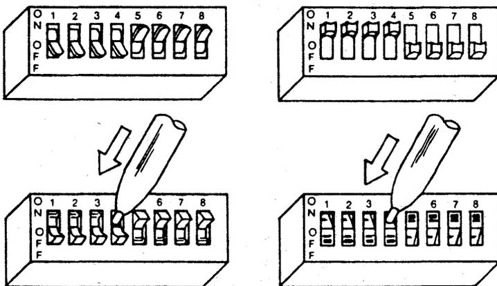
Figure 25: Setting Slide and Rocker Switches
