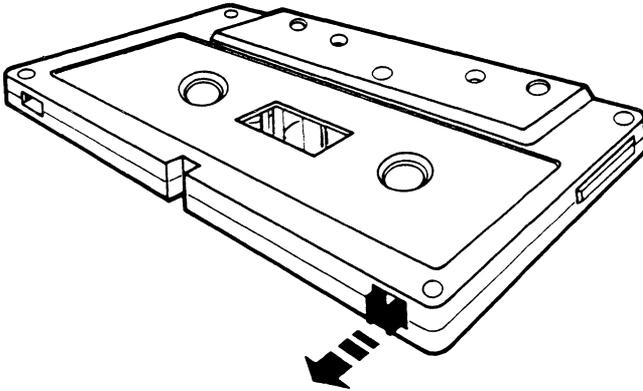
**Figure 3-25.** Write Enabling/Protecting a Cassette Tape
