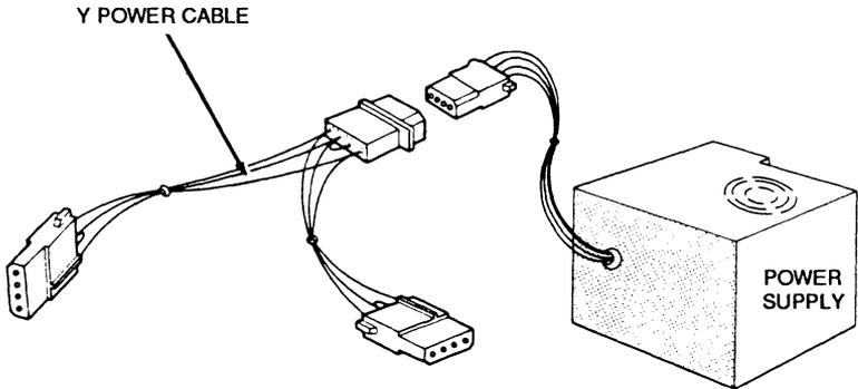
**Figure 2-1** Adding a Y Power Cable
