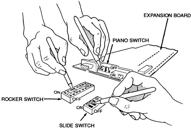
**Figure 3-26.** Setting Slide and Rocker Switches
