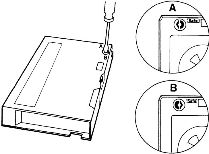
**Figure 3-24.** Write Enabling/Protecting a Cartridge Tape
