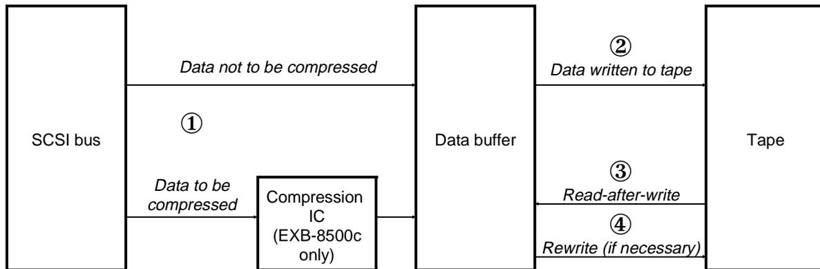
Figure 5-1 Data flow during a write operation
