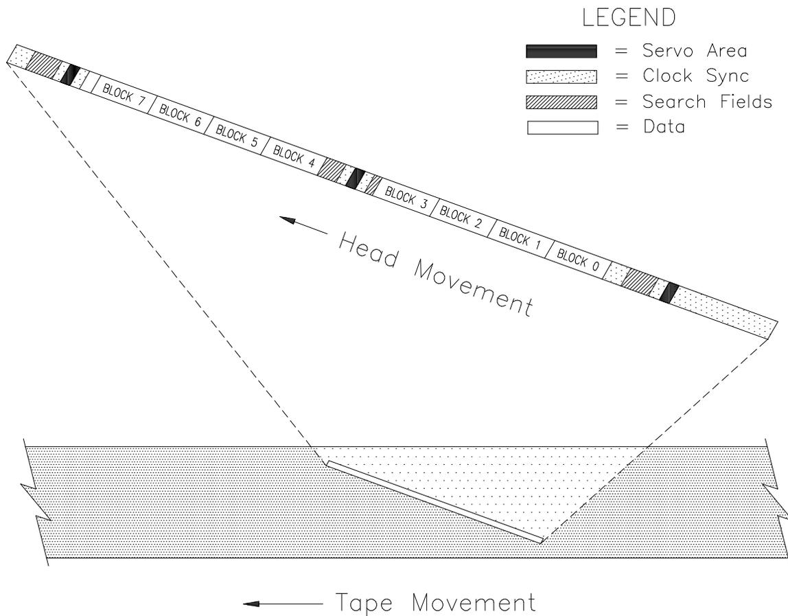
Figure 4-4 Physical track structure for EXB-8200c track format
