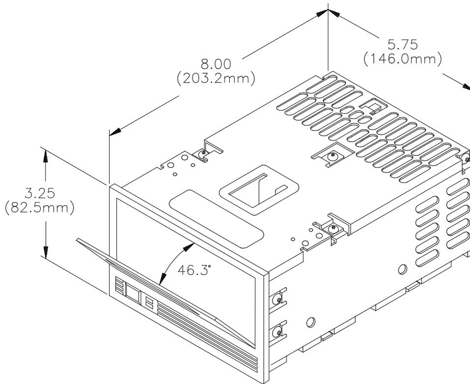
Figure 2-3 External dimensions in inches (and millimeters)
