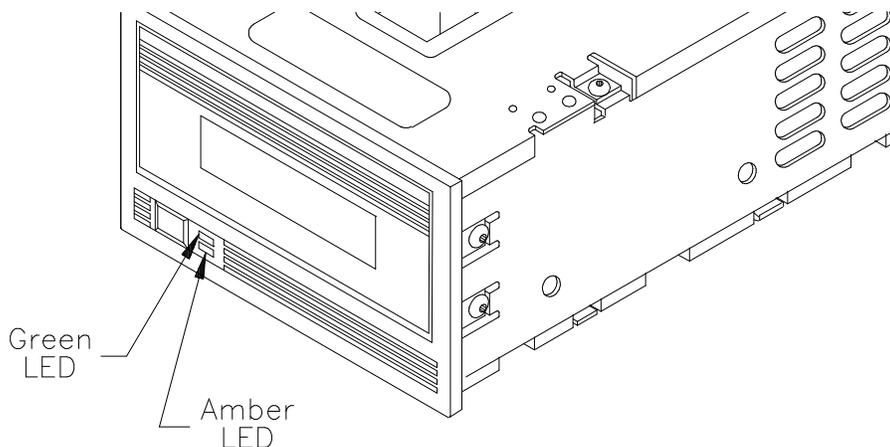
Figure 12-1 LEDs on the front of the EXB-8500
