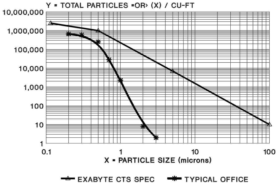
Figure 9-2 Particulate contamination specification vs. typical office
