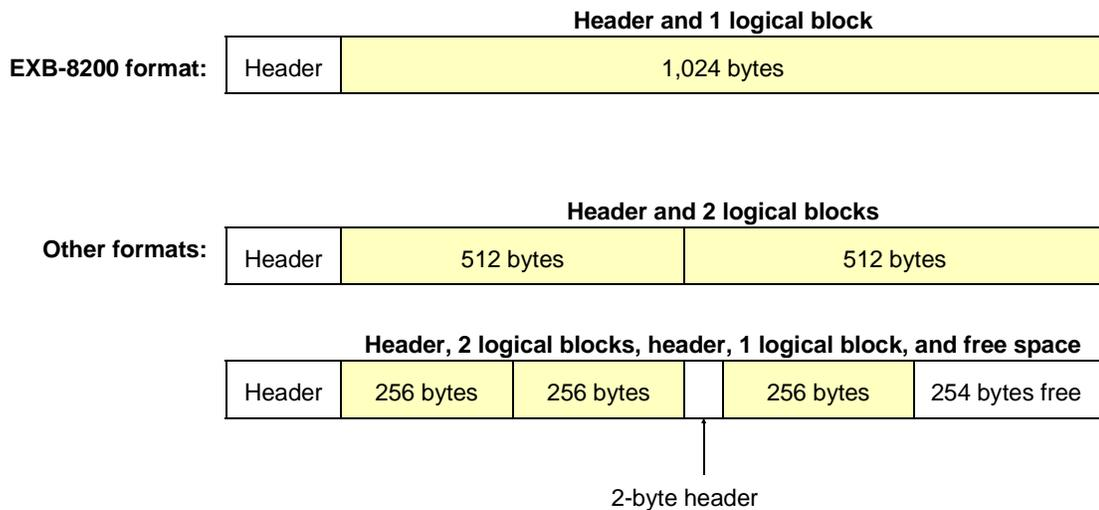
Figure 4-7 Logical block packing (one physical block)
