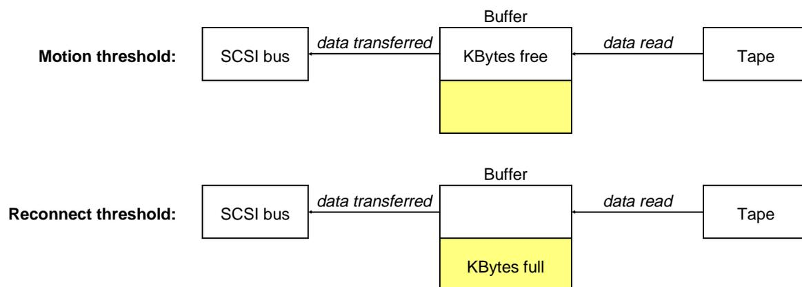
Figure 5-5 Motion and reconnect thresholds during a read operation
