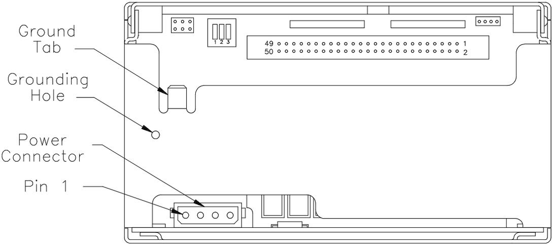
Figure 8-1 Power connector and ground (single-ended configuration)
