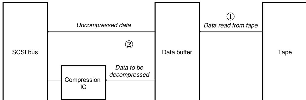
Figure 5-4 Data flow during a read operation
