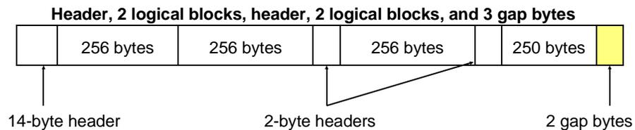
Figure 4-8 Gap bytes (one physical block)
