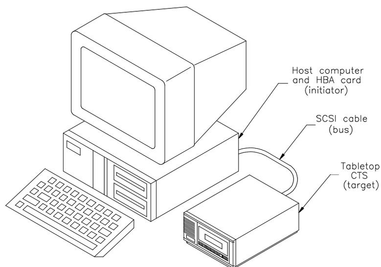
Figure 3-1 Physical connection in the SCSI environment (example)
