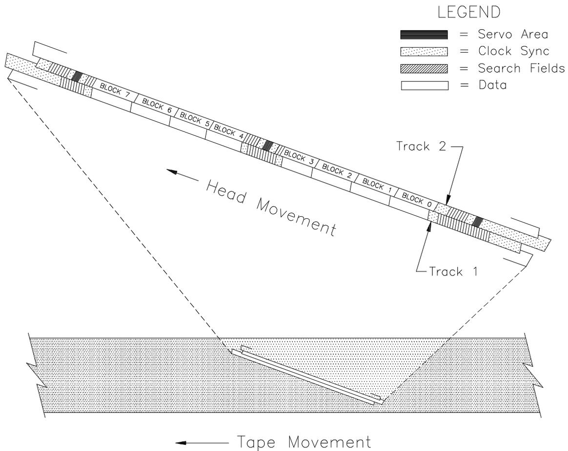
Figure 4-2 Physical track structure for EXB-8500/EXB-8500c format
