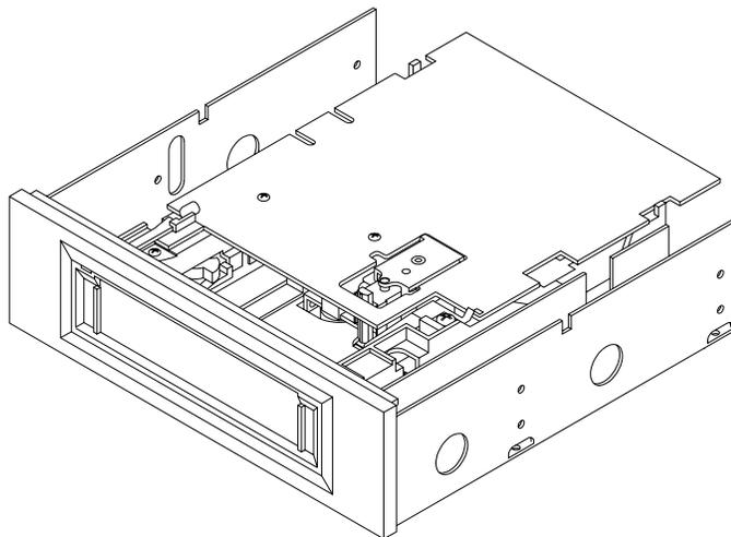
The Eagle TR-3 is a minicartridge tape drive that interfaces directly with a floppy controller in a computer. When used with backup software, this tape drive is ideally suited for system backup and restore tasks in a desktop PC environment. The Eagle TR-3 can store up to 4.2 gigabytes of data on a single minicartridge (depending on the cartridge type and assuming a software data compression ratio of 2:1).
