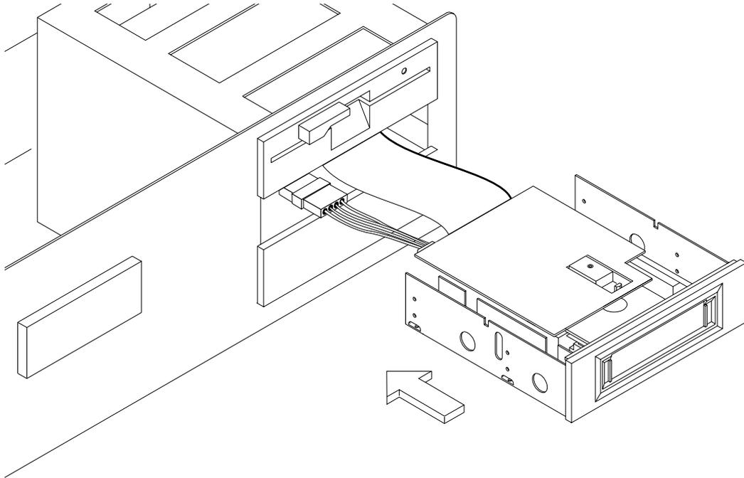
The tape drive is shipped with mounting hardware that extends it to a 5.25-inch, half-high form factor. If you want to use the tape drive in a 3.5-inch, one-inch form factor, remove the mounting hardware.
