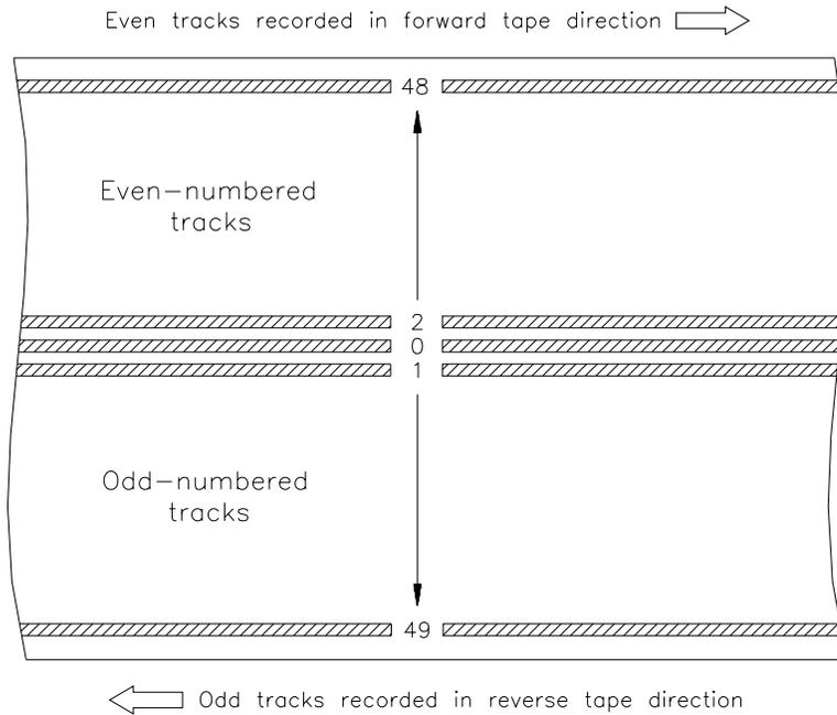
The tape drive records 50 tracks of data on the TR-3, QIC-Wide, and QIC-EXtra 8mm minicartridges. For the MC3000XL and QIC-EXtra quarter-inch minicartridge, it records 40 tracks.
