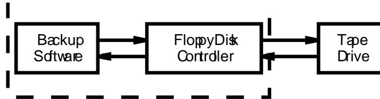
1. When your backup software issues a command to the tape drive, the command is sent to the floppy controller in the host computer.
