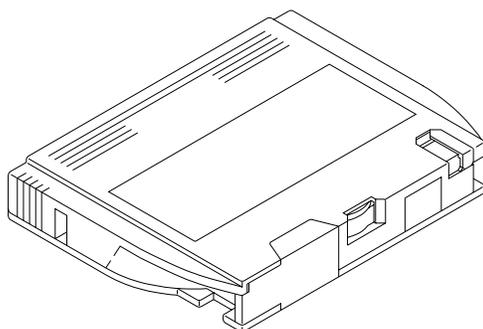
**Note:** With the appropriate software, the tape drive can read (but not write) TR-1, QIC-80, and QIC-40 formatted tapes.
