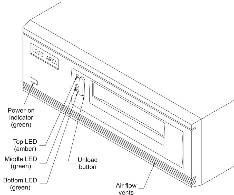
**Figure A-2** Front panel of the tabletop tape drive
