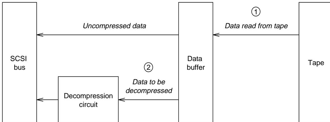
**Figure 3-2** Data flow during a read operation
