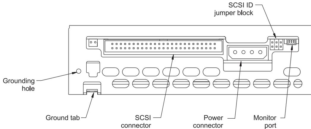
**Figure 1-4** Back panel of the internal tape drive
