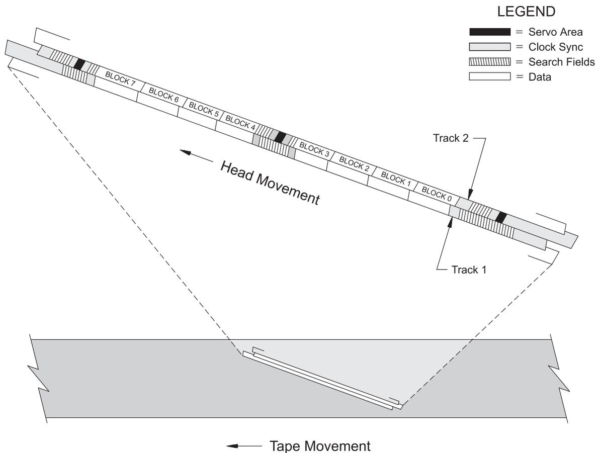
**Figure 2-2** 8500/8500c physical track structure
