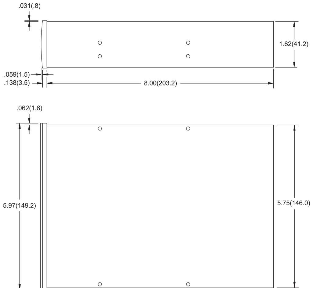
**Figure 1-7** Dimensions of the internal tape drive in inches (and mm)
