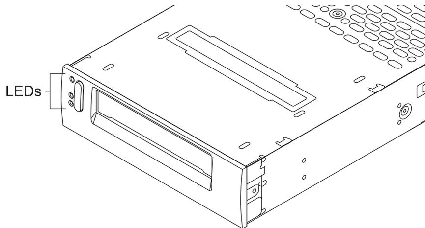
Figure 4-8 Tape drive LEDs
