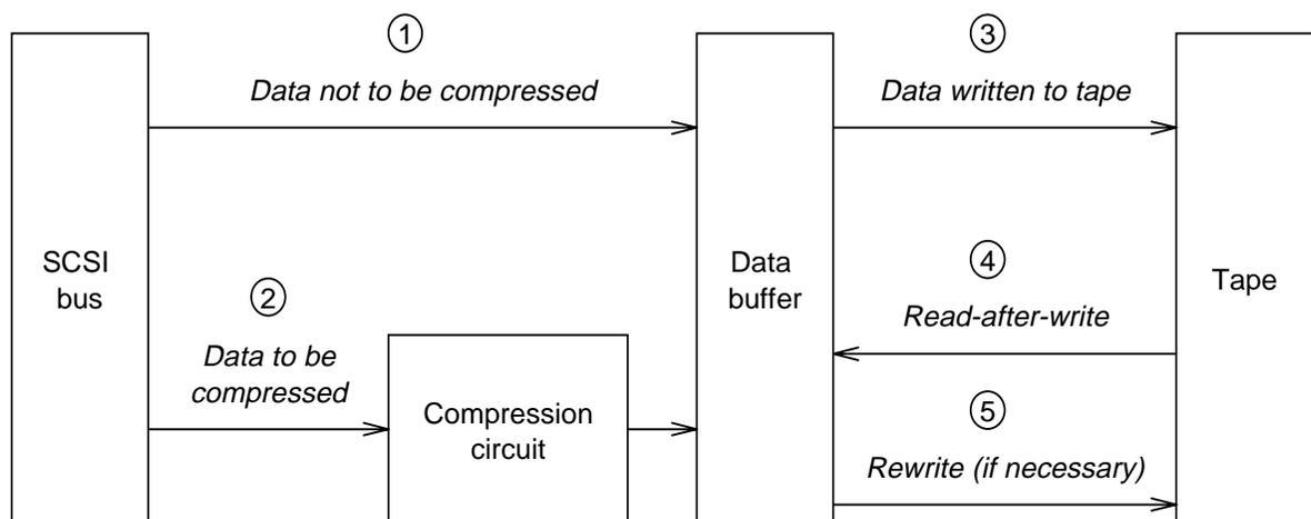
**Figure 3-1** Data flow during a write operation
