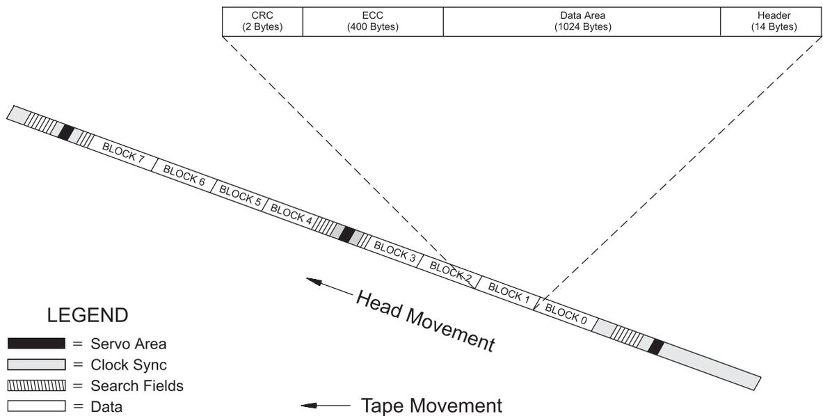
**Figure 2-4** Physical block format
