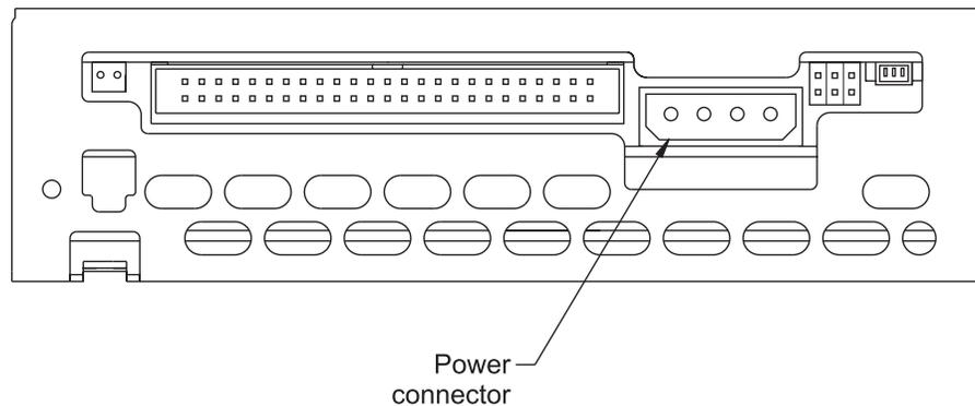
**Figure 4-6** Power connector on the back of the internal tape drive
