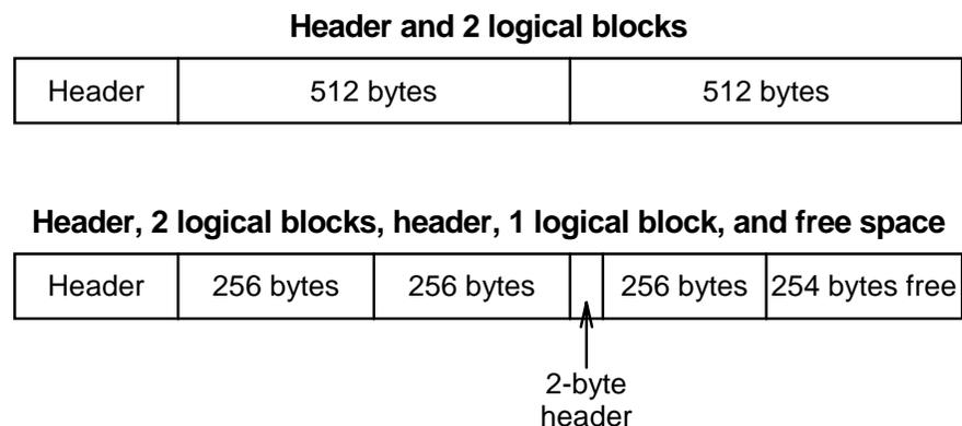
**Figure 2-5** Logical block packing in one physical block
