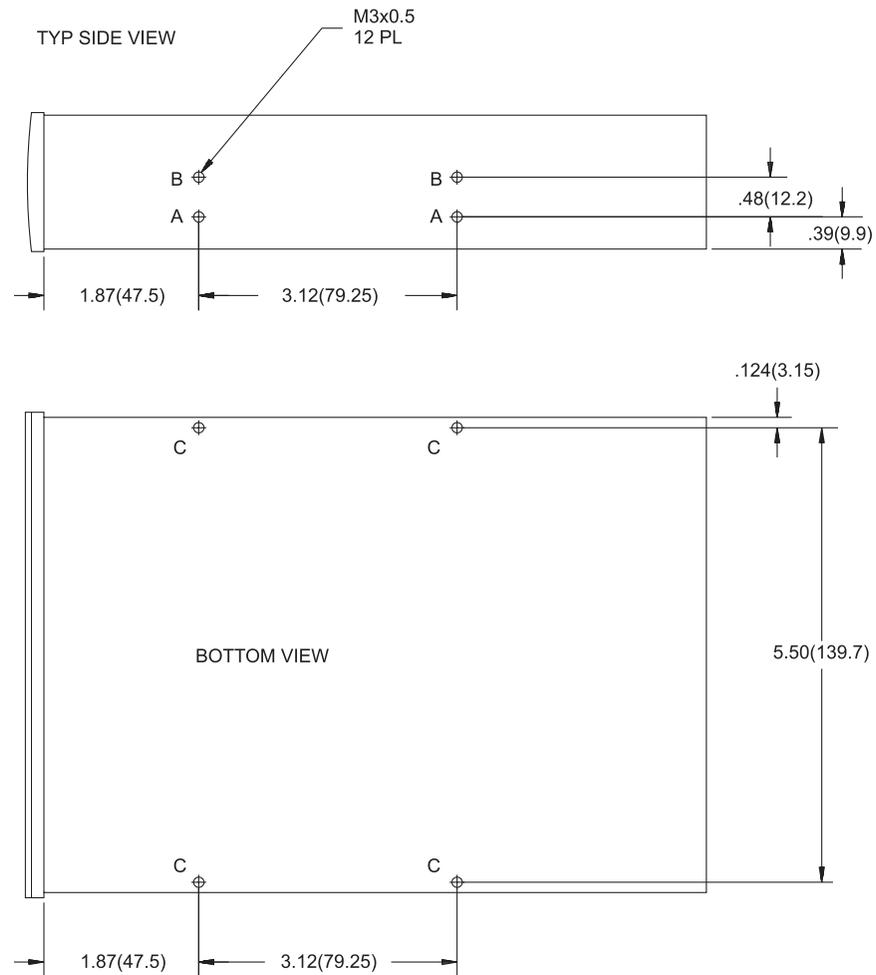
Figure 4-4 Mounting hole dimensions in inches (and mm)
