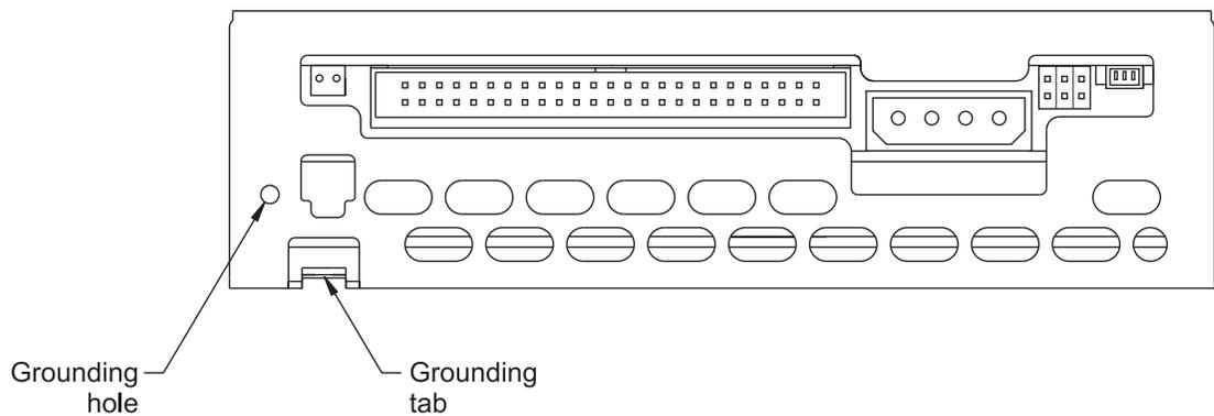
**Figure 4-7** Chassis grounding points on the internal tape drive
