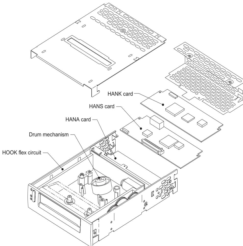
**Figure 1-5** Internal components
