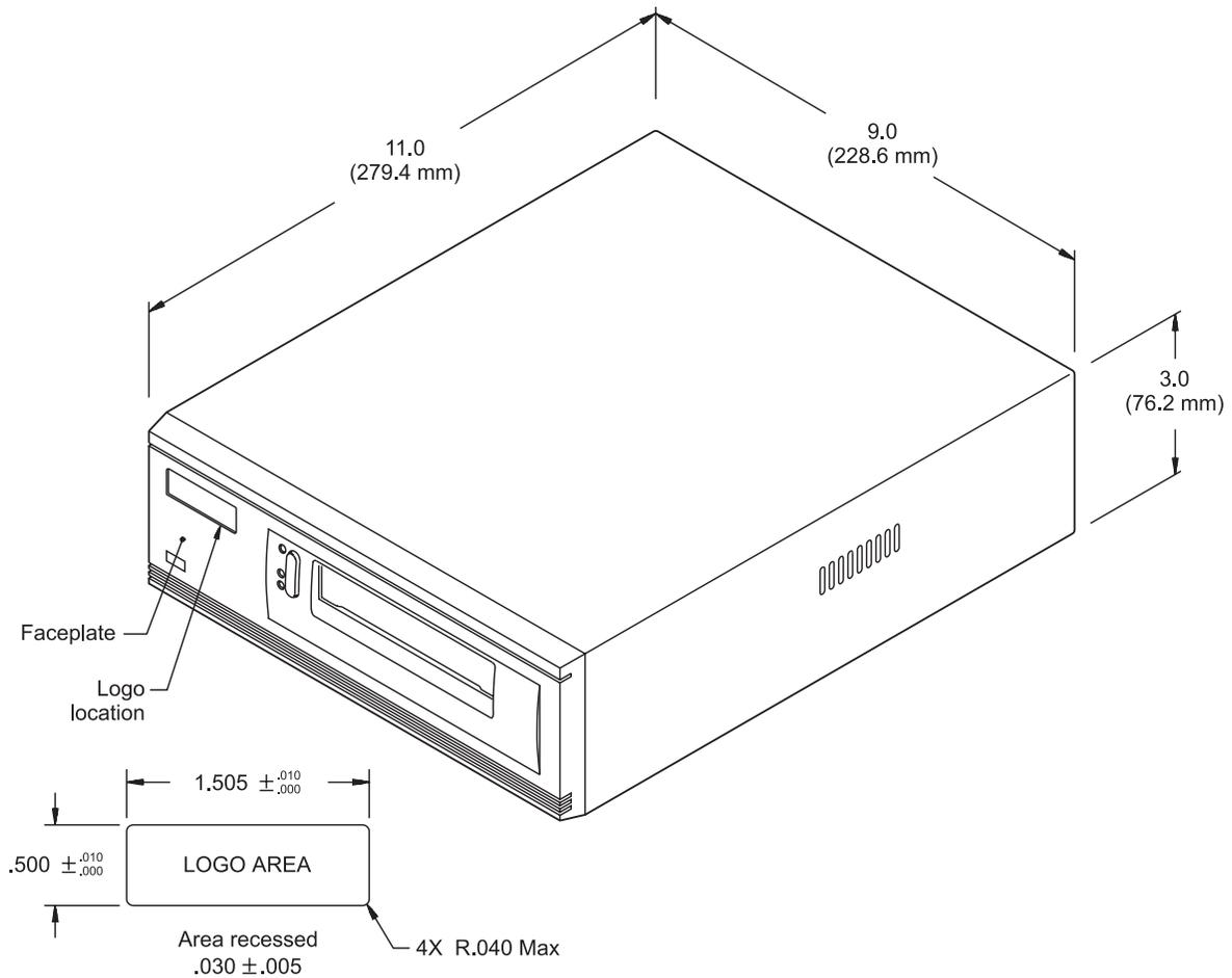
Figure A-5 Dimensions of the tabletop tape drive in inches (and mm)
