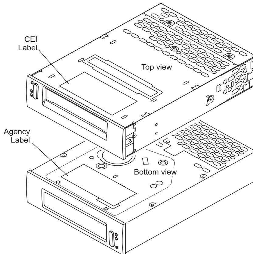
**Figure 1-3** Labels on the internal tape drive
