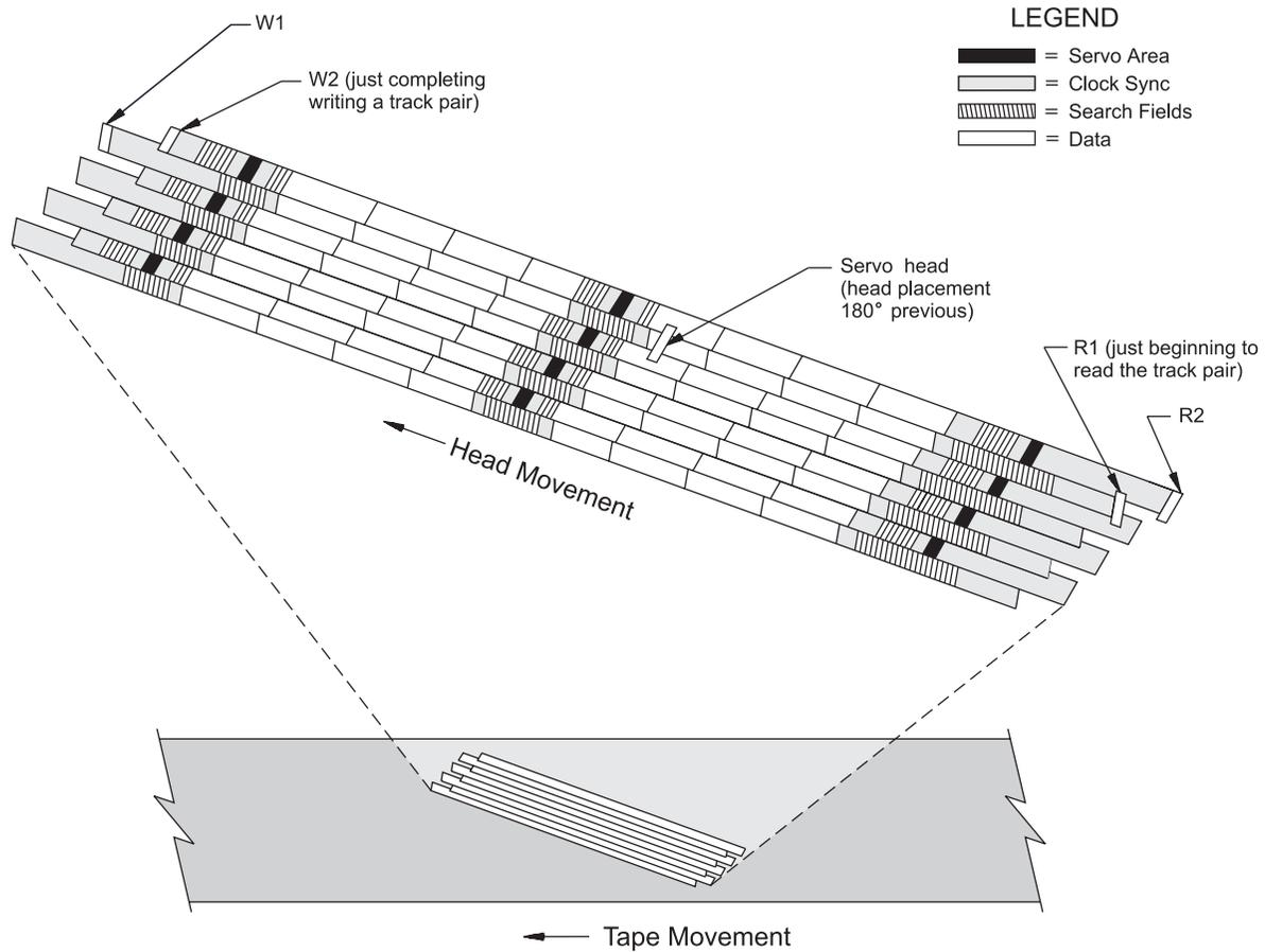
**Figure 2-3** Position of the tape drive's heads relative to the tracks (8500/8500c format)
