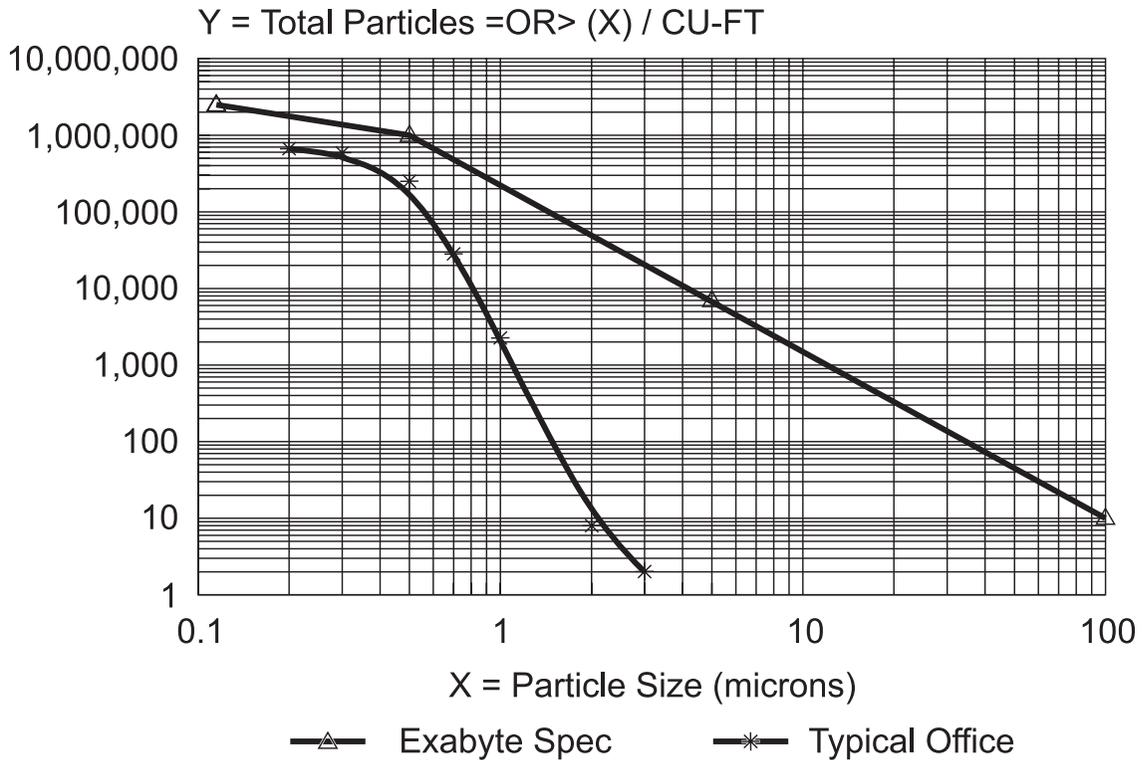
Figure 6-2 Particulate contamination specification vs. typical office
