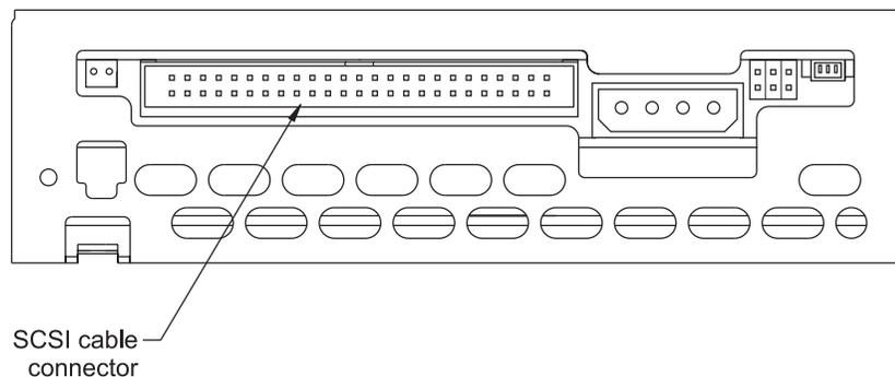
**Figure 4-5** SCSI connector on the back of the internal tape drive
