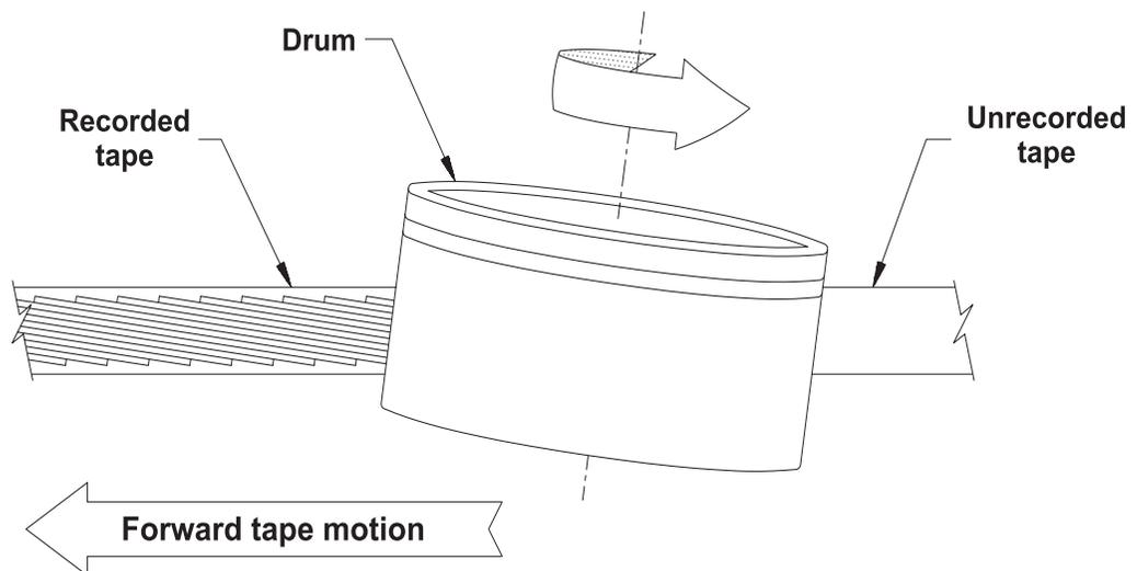
Figure 2-1 Helical-scan recording
