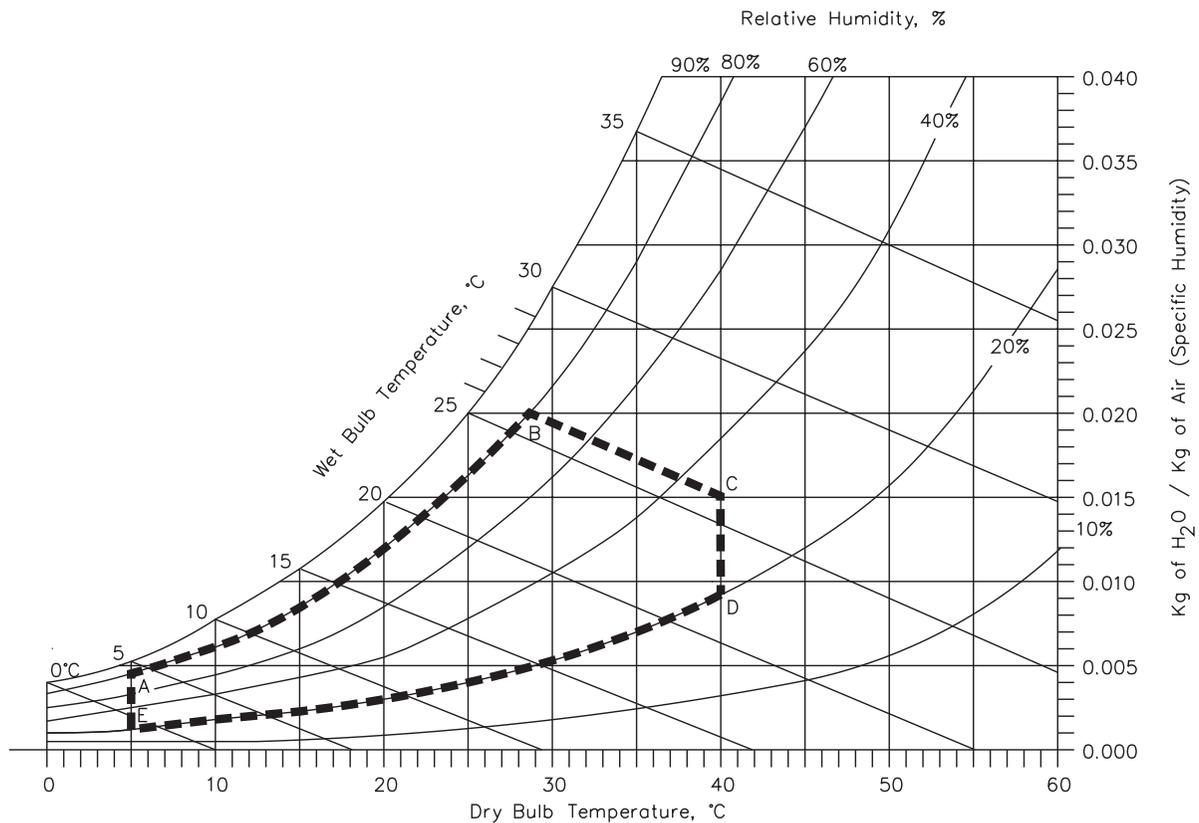
**Figure 6-1** Tape path temperature and humidity ranges for operation
