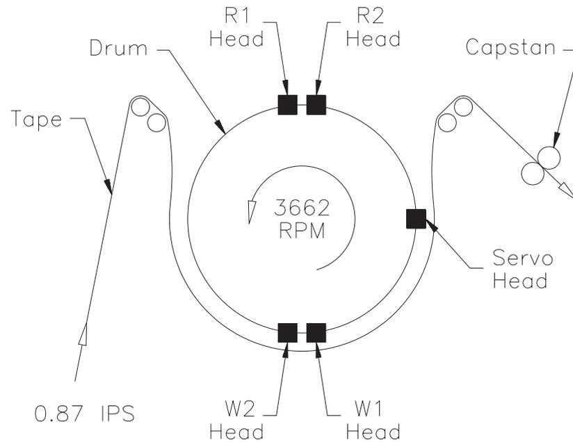
**Figure 1-6** Location of the heads on the drum mechanism
