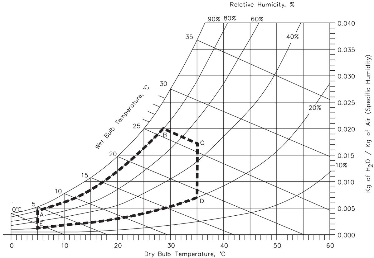
**Figure A-6** Ambient operating environment for the tabletop tape drive
