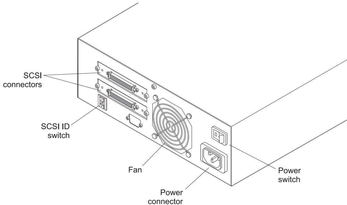
**Figure A-3** Back panel of the tabletop tape drive
