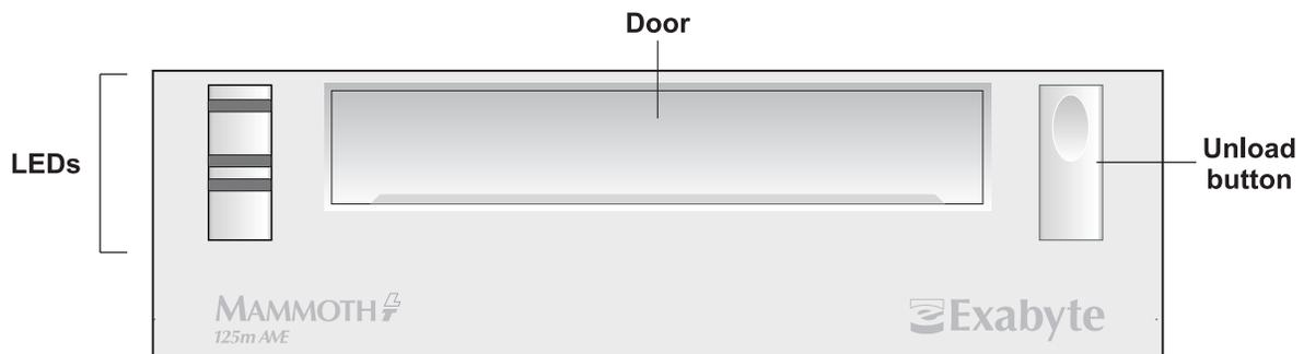
Figure 2-8 Front panel controls and indicators
