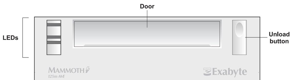
**Figure 1-3** Front panel components
