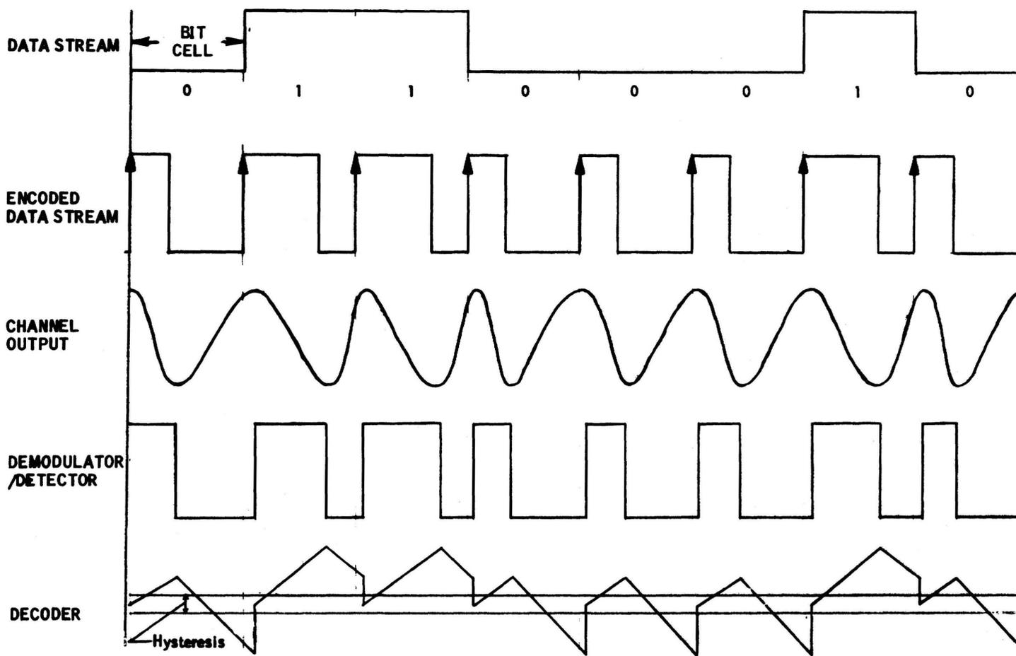
FIGURE 5. A speed-insensitive, data-encoding scheme called ratio recording. The first line is the incoming data; the second is the encoder output; the third is the playback signal; the fourth is the demodulated signal. The bottom line is the data decoded by integrating positively from the clock transition to the data transition and negatively to the next clock transition.
