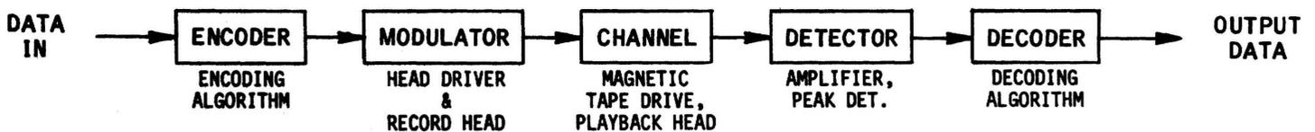
THE ELEMENTS IN A TAPE SYSTEM ANALOG TO A COMMUNICATIONS CHANNEL.
