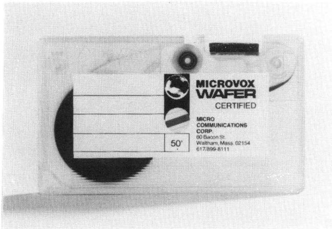
FIGURE 1. Endless-loop magnetic tape wafer cartridge (full size).
