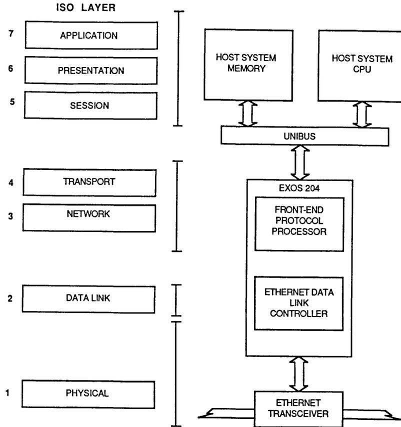
Figure 1-1: The EXOS 204 Front-End Mode Implementation and ISO/OSI
