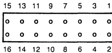
**Figure C-1: Pin Layout for Transceiver Connector on EXOS 204**
