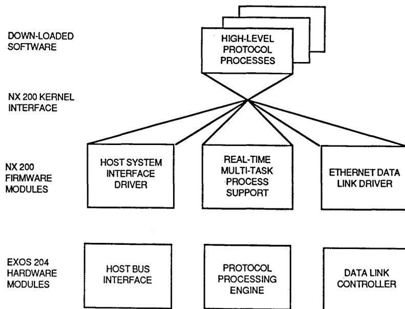
Figure 1-3: NX 200 Software Architecture
