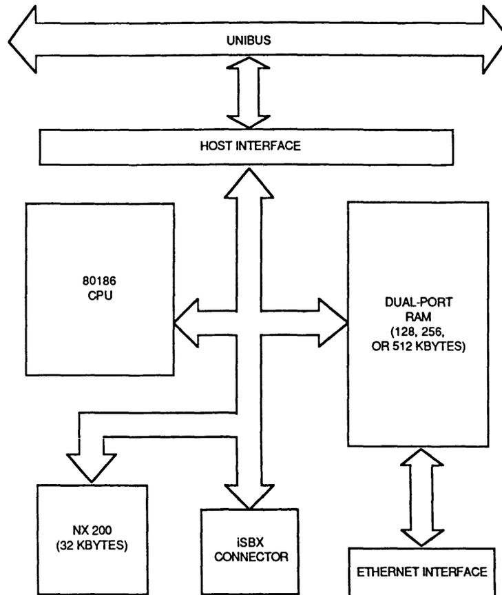
Figure 1-2: EXOS 204 Block Diagram
