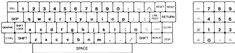
**Figure 3. The Keyboard (Characters without Shifting)**
