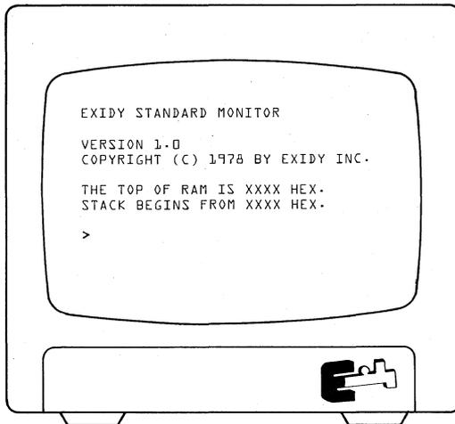
Without a ROM PAC inserted into the side of Sorcerer, the internal Power-On Monitor program is automatically executed and the above message displayed.
