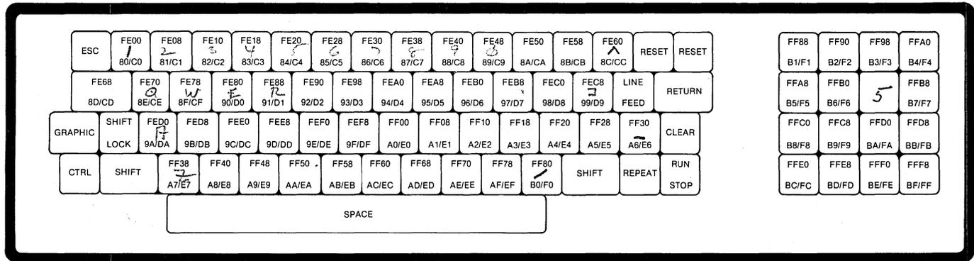
**Figure 8. User Graphic Storage Addresses and ASCII numbers**
