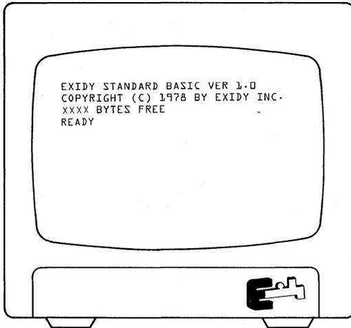
With a ROM PAC inserted correctly into the side of Sorcerer, you will see a ROM PAC sign-on message on the screen. This is the Standard BASIC signature.
