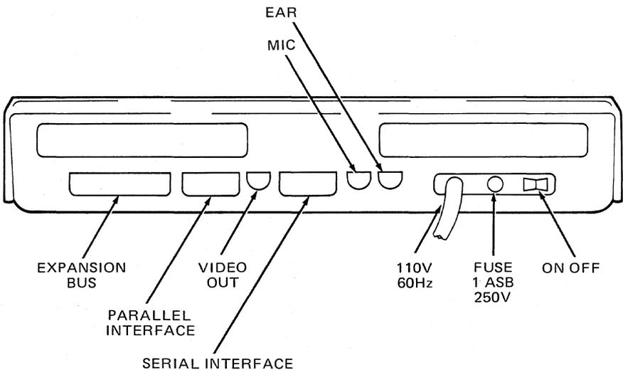
**Figure 1. Connector Locations at the Back of Sorcerer**
