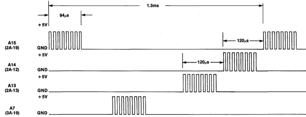
**Figure 11. Data-Out Line Waveforms (Program 2)**
