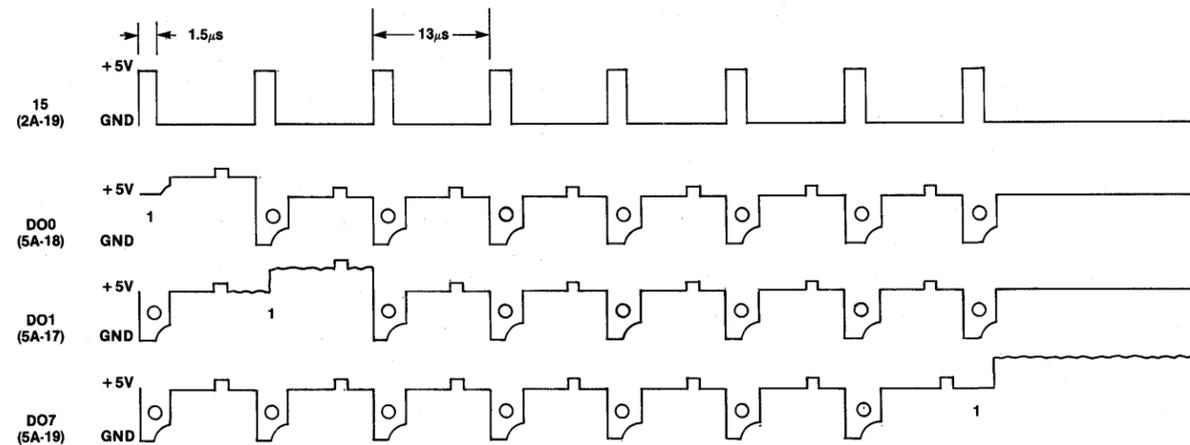
**Figure 12. Data-In Line Waveforms (Program 3)**
